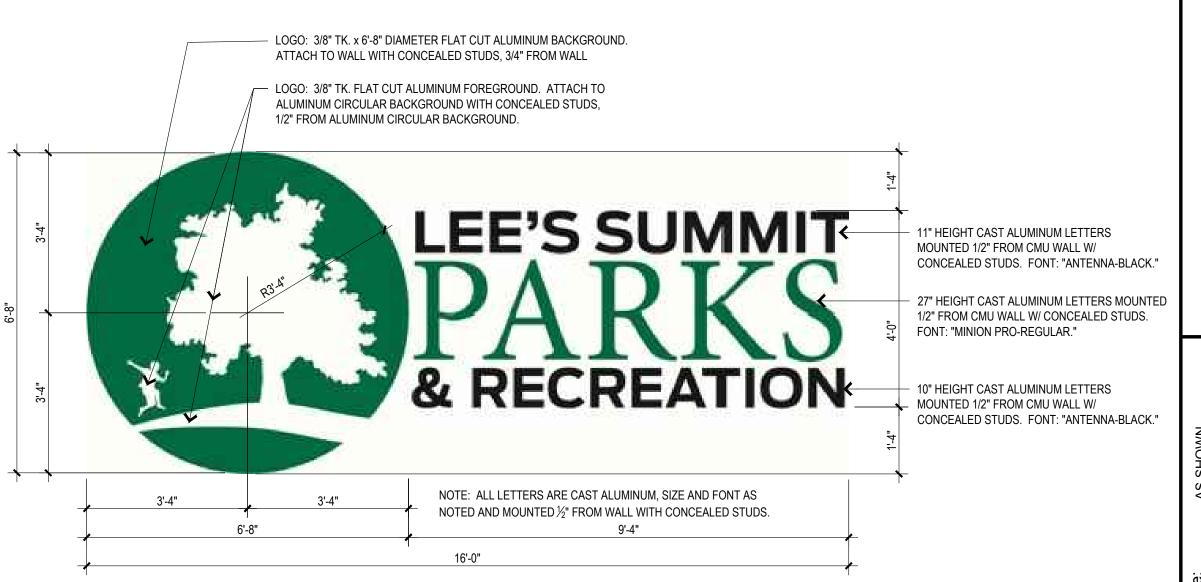
8 DETAIL ELEVATION - SIGNAGE ON BUILDING ABOVE WAVEPOOL
