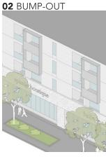
PROTRUDING ELEMENTS ON THE FACE OF A BUILDING TO PROVIDE ADDITIONAL RELIEF.
