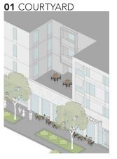
LARGE SETBACKS USED TO PROVIDE RELIEF ON A LONG FACADE.
