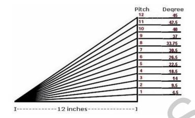
This drawing demonstrates how many degrees rise for each pitch of a typical roof. Look at the column labeled pitch, then look under degrees to get the corresponding amount of degrees. Example: 3/12 pitch = 14 degrees.
