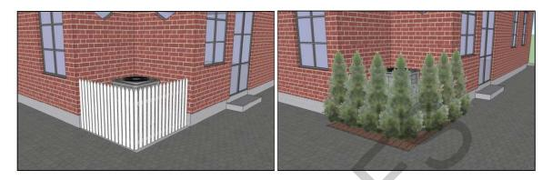
HVAC units and condensers at rear facades shall be screened through fencing or landscaping. Units should have 36 inches of clearance to allow for maintenance and servicing.
