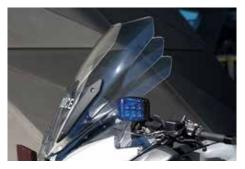
The windshield is electrically adjustable to continuously variable levels and reduces noise levels to a minimum.
