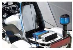
Analog and digital radio end devices can be used at the same time and are securely stowed in the electrically unlockable radio box.
