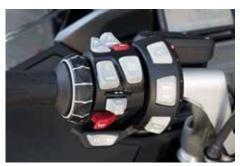
Newly developed additional switch units include freely programmable keys for special functions. The logically arranged controls ensure simply handling.
