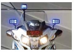
The LED flashlight and rotating beacon with telescopic rod can be controlled separately at the front and rear. The LED display can be programmed to show "Stop" or "Please follow".
