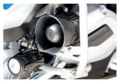
Enhanced safety is ensured by the speedrelated volume of the acoustic signal system and the supplementary headlamp.
