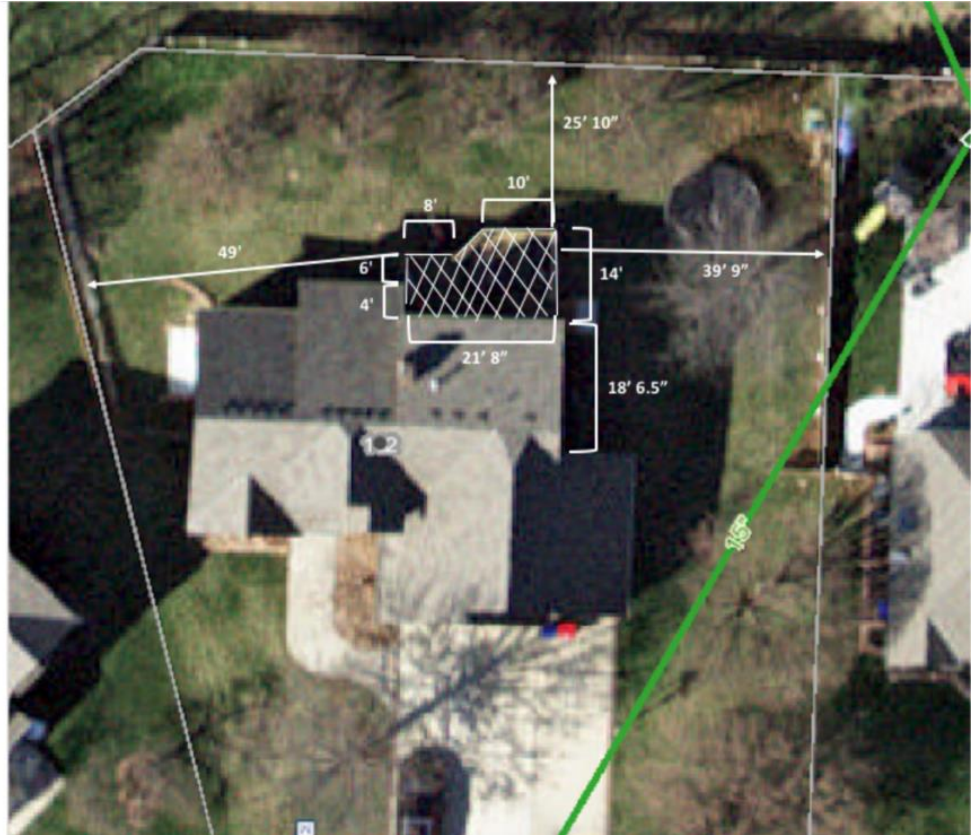
Figure 2 – Existing uncovered deck (with dimensions).
