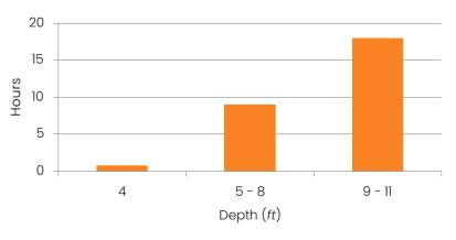
Figure 3: Hours Required in Relation to Pipe Depth
