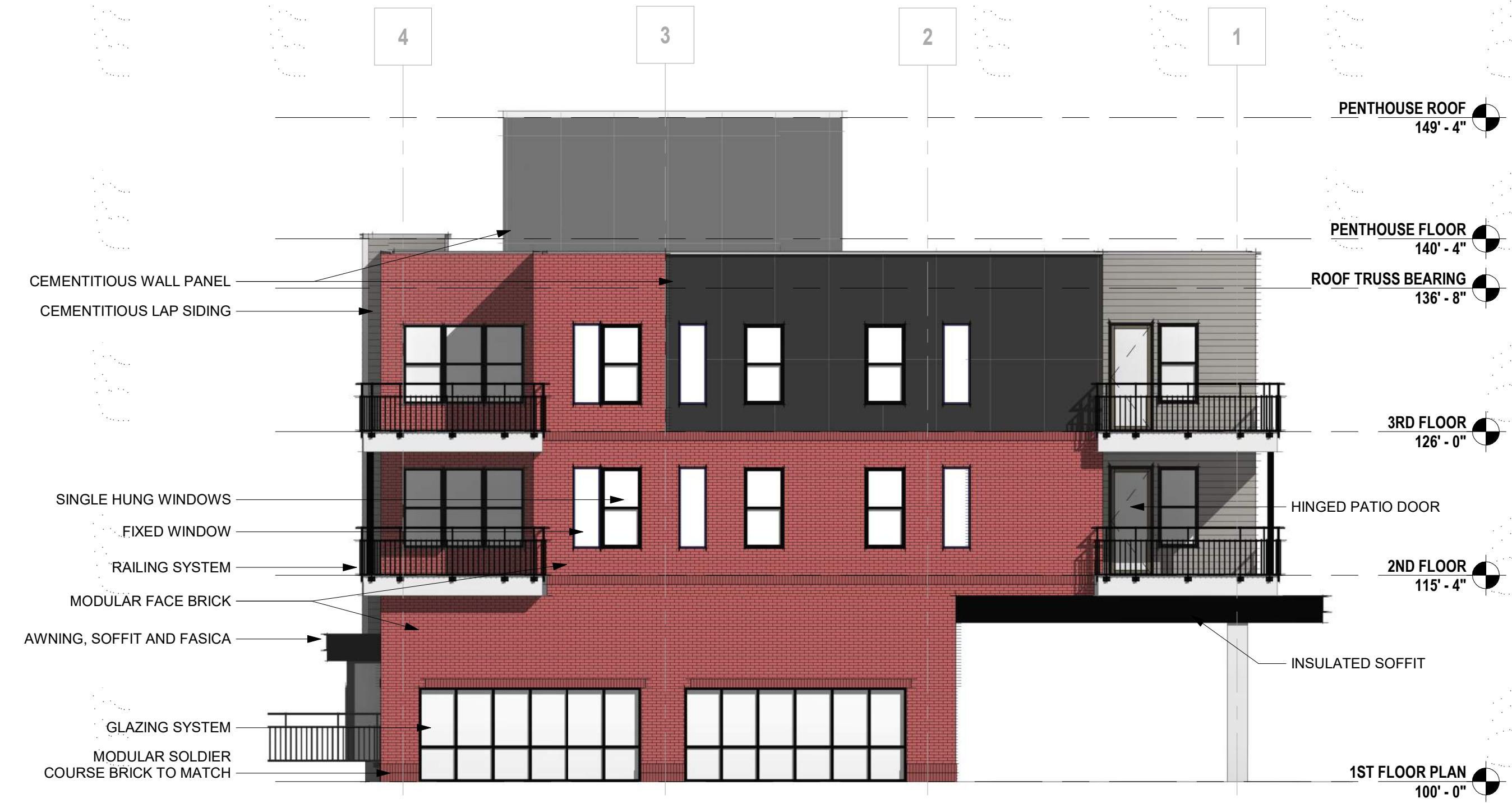
E5 ELEVATION - NORTH 1/8" = 1'-0"
