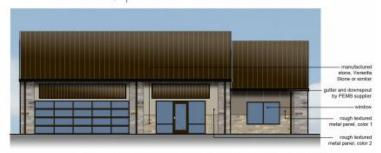
7 East Elevation (exterior facing) - Bldg 1
