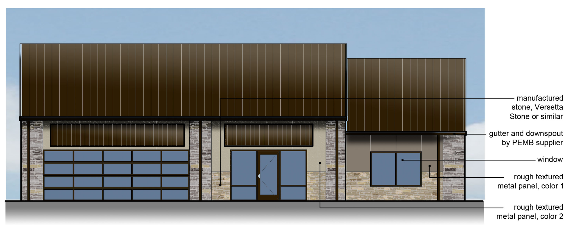
7 East Elevation (exterior facing) - Bldg 1 scale: 1/8" = 1'-0"
