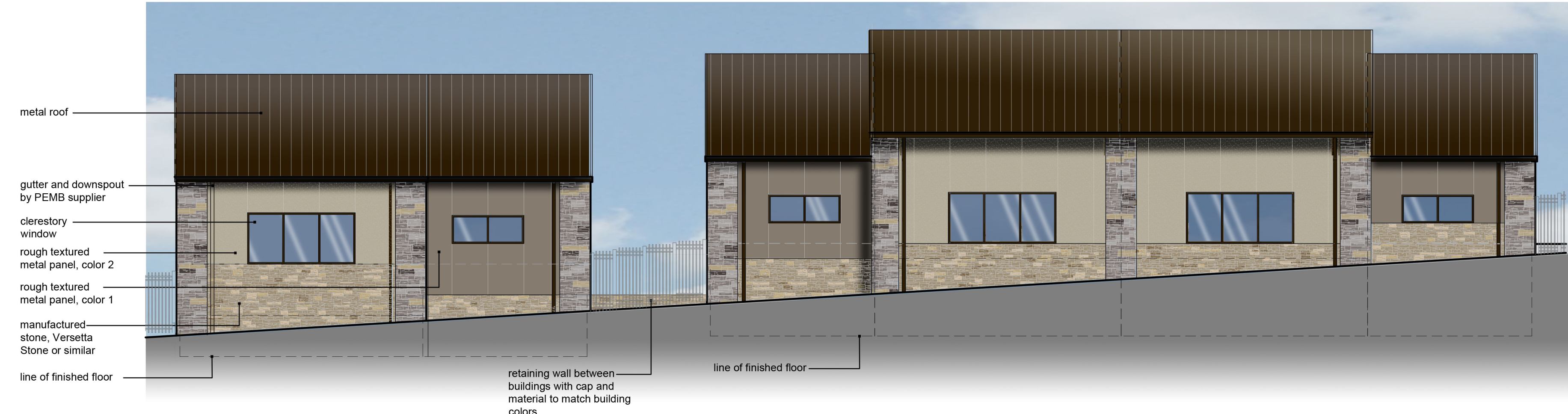
2 South Elevations (facing Strother) - Bldg 8 scale: 1/8" = 1'-0"
