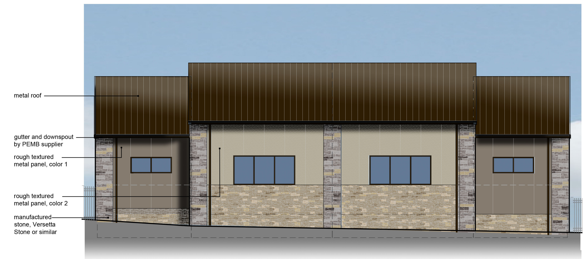
3 North Elevation (exterior facing) - Bldg 19, 20 scale: 1/8" = 1'-0"
