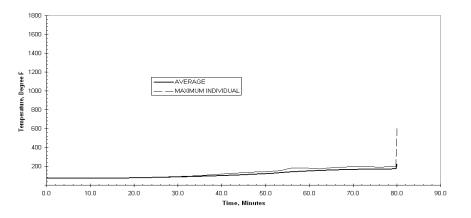
Figure 67 – Plot of Temperatures of the Unexposed Surface vs. Time for Test Assembly No. 8
