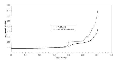
Figure 10 - Plot of Temperature of the Top of Subfloor vs. Time for Assembly No. 1
