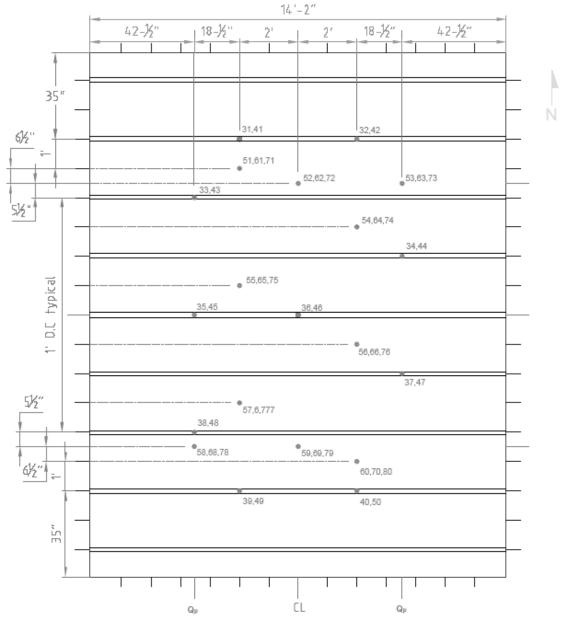
Figure A.4.4 – Thermocouple Locations on Wood Members.
