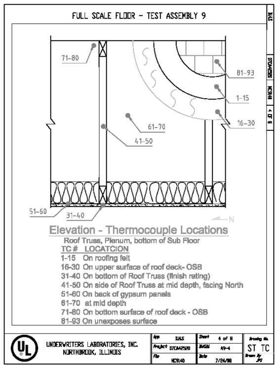
Figure A.9.3 – Thermocouple Locations - Elevation.
