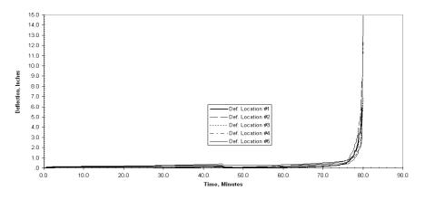
Figure 68 – Plot of Deflections vs. Time for Test Assembly No. 8
