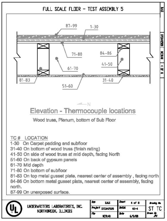
Figure A.5.3 – Thermocouple Locations - Elevation.
