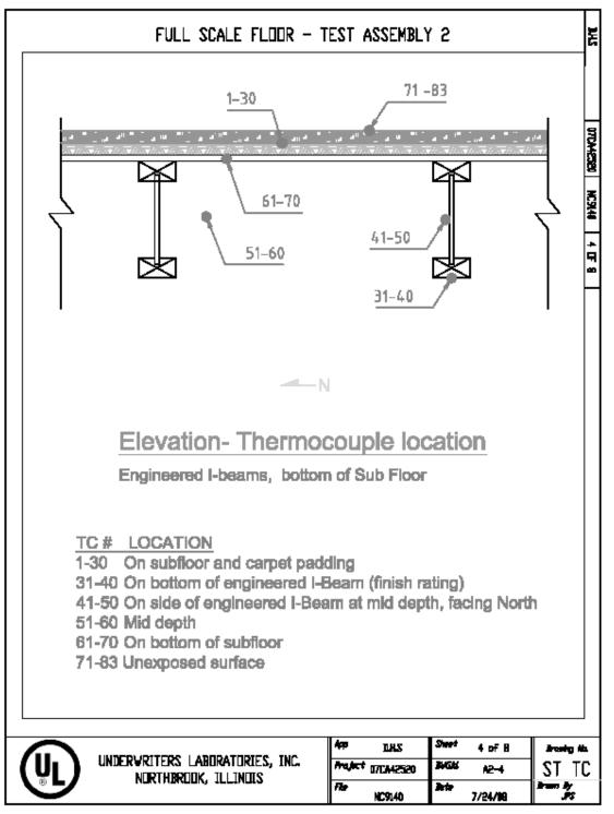
Figure A.2.3 – Thermocouple Locations - Elevation.
