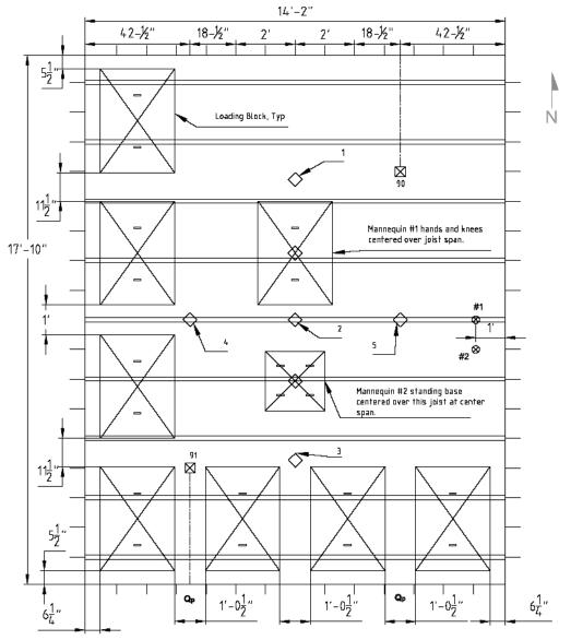
Figure A.2.7 – Loading and Instrumentation Layout (See Figure A.2.8).
