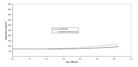
Figure 12 - Plot of Unexposed Surface Temperatures vs. Time for Assembly No. 2
