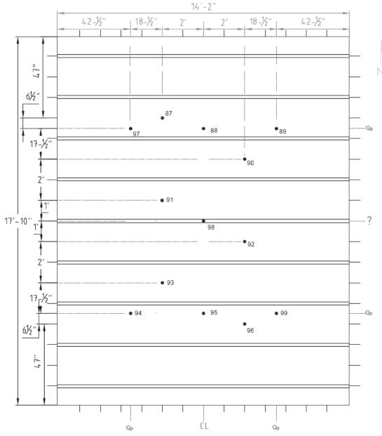
Figure A.5.6 – Thermocouple Locations on Unexposed Surface.
