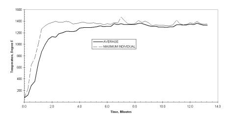
Figure 40 – Plot of Temperatures of the Top Metal Gusset Plates vs. Time for Assembly No. 3
