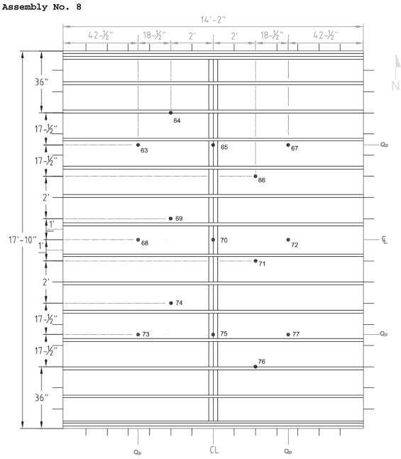
Figure A.8.6 – Thermocouple Locations on Unexposed Surface.
