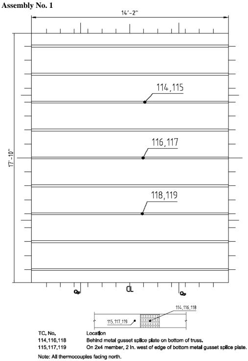
**Figure A.1.8 – Thermocouple Locations on Metal Gusset Plates**
