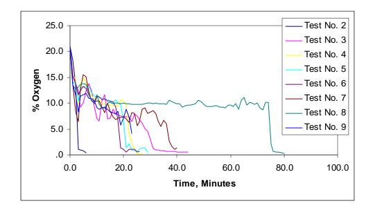
Figure 79 - Percent Oxygen in Furnace
