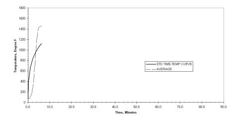
Figure 6 – UL263 Standard Time Temperature Curve and Average Furnace Temperature vs. Time for Assembly No. 2
