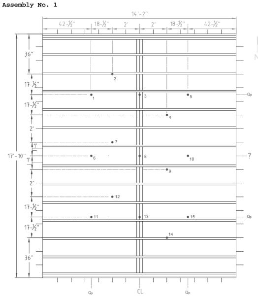
Figure A.1.5 – Thermocouple Locations on Subfloor.
