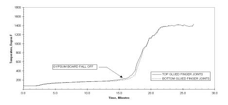
Figure 45 - Plot of Temperature of the Top and Bottom Glued Finger Joints vs. Time for Assembly No. 6
