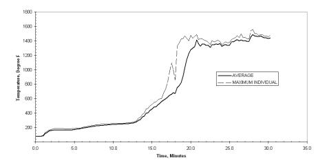
Figure 9 - Plot of Temperature of the Unexposed Surface of Gypsum Board vs. Time for Assembly No. 1
