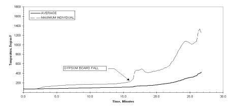
Figure 47 - Plot of Temperature of the Subfloor Temperatures vs. Time for Test Assembly No. 6
