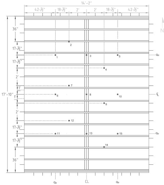
Figure A.8.5 – Thermocouple Locations on Subfloor.
