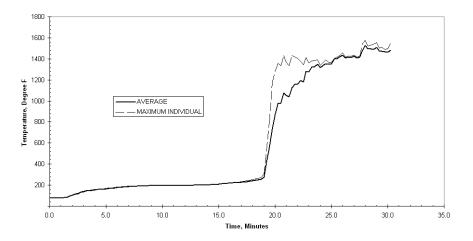
Figure 17 - Plot of Temperatures of the Truss Splice Behind Connection of Metal Gussets vs. Time for Assembly No. 1
