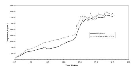
Figure 13 - Plot of Temperatures over the Can Lights vs. Time for Assembly No. 1
