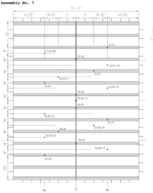
Figure A.7.4 – Thermocouple Locations on Wood Members.
