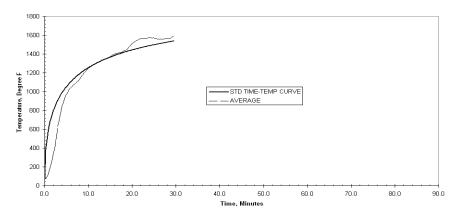
Figure 31 - UL263 Standard Time Temperature Curve and Average Furnace Temperature vs. Time for Assembly No. 5
