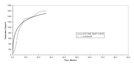
Figure 41 - UL263 Standard Time Temperature Curve and Average Furnace Temperature vs. Time for Assembly No. 6
