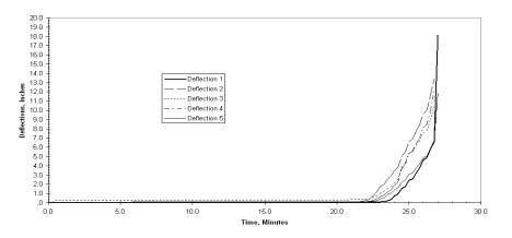
Figure 30 - Plot of Deflections vs. Time for Assembly No. 4
