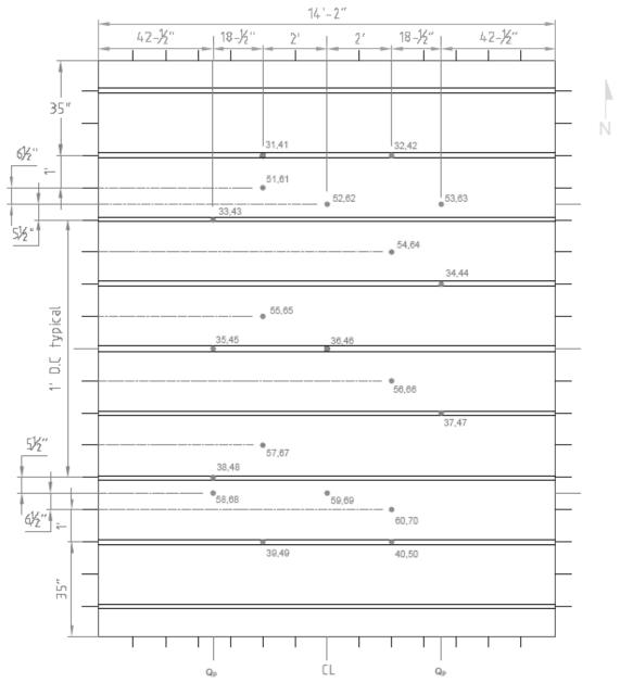
Figure A.2.4 – Thermocouple Locations on Wood Members.
