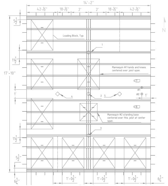
Figure A.3.7 – Loading and Instrumentation Layout (See Figure A.3.8).
