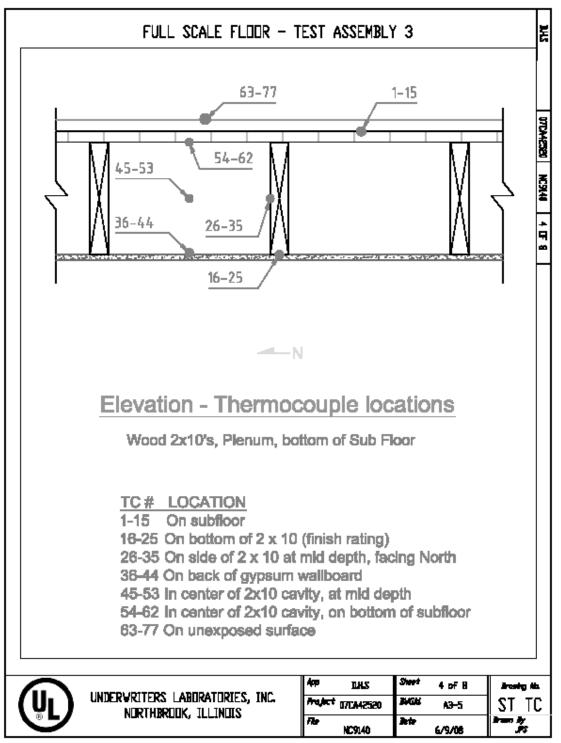
Figure A.3.3 – Thermocouple Locations - Elevation.
