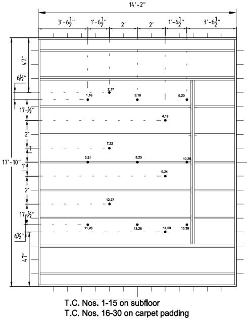
Figure A.3.5 – Thermocouple Locations on Subfloor and on Carpet Padding.
