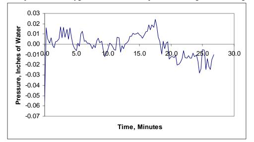
The furnace pressure and oxygen concentration are presented in Figure 42 and Figure 43.
