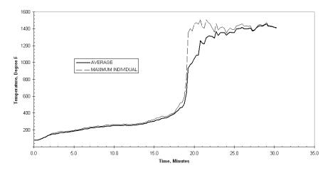
Figure 16 - Plot of Temperatures over the Rigid Duct vs. Time for Assembly No. 1
