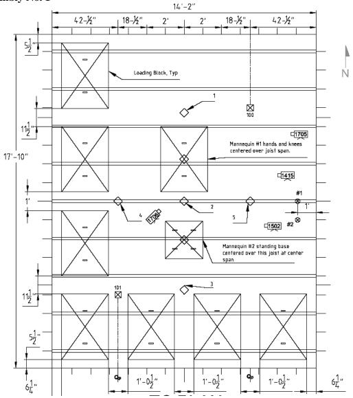
Figure A.1.9 – Loading and Instrumentation Layout (See Figure A.1.10).
