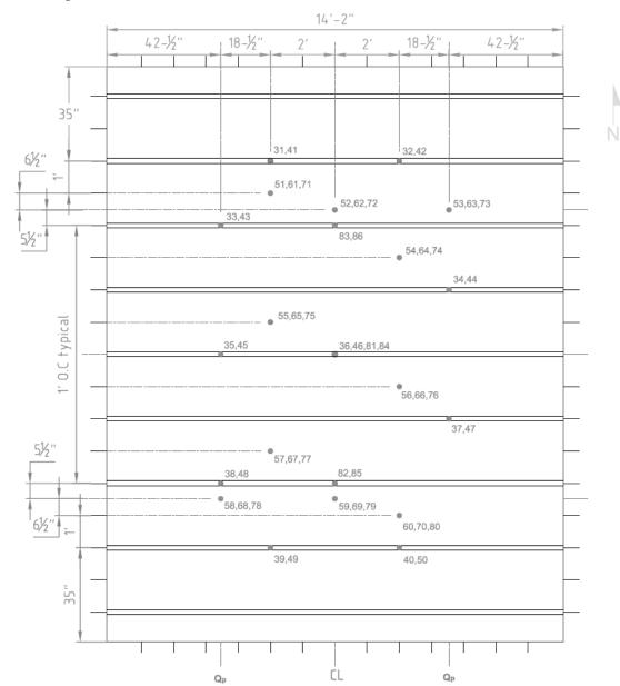
Figure A.6.4 – Thermocouple Locations on Wood Members.
