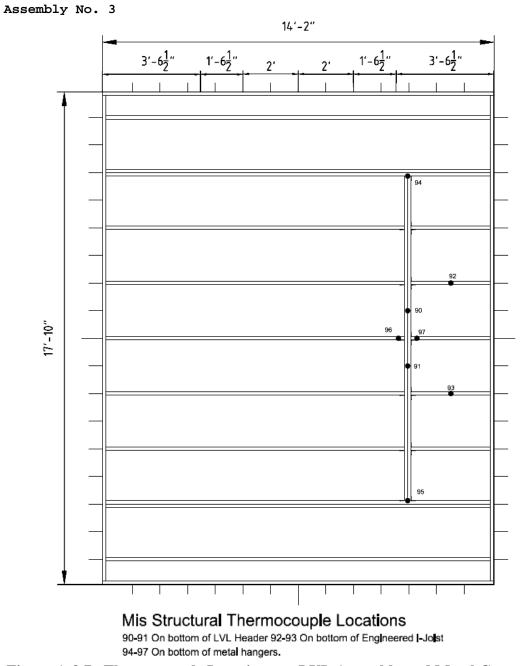
Figure A.3.7 – Thermocouple Locations on LVL Assembly and Metal Connectors.
