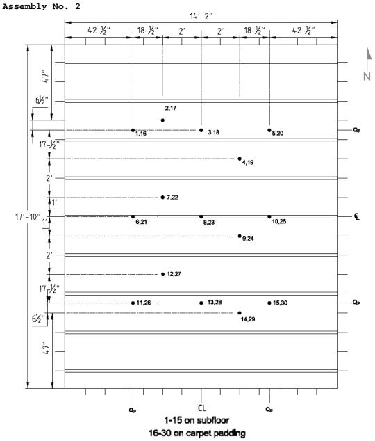
Figure A.2.5 – Thermocouple Locations on Subfloor and Carpet Padding.
