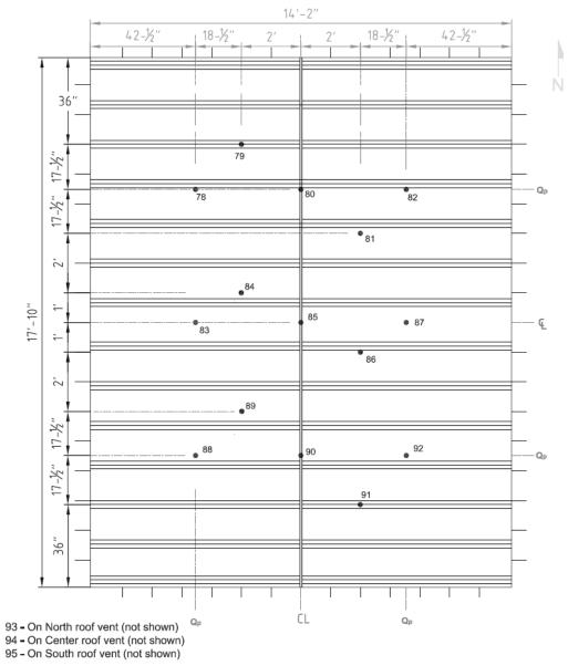
Figure A.7.6 – Thermocouple Locations on Unexposed Surface.
