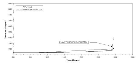
Figure 39 - Plot of Temperatures of the Unexposed Surface vs. Time for Assembly No. 5
