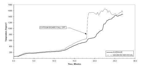
Figure 26 - Plot of Temperature of the Unexposed Surface of Gypsum Board vs. Time for Assembly No. 4
