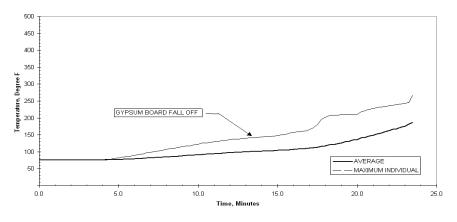
Figure 74 – Plot of Temperature of the Roofing Felt vs. Time
