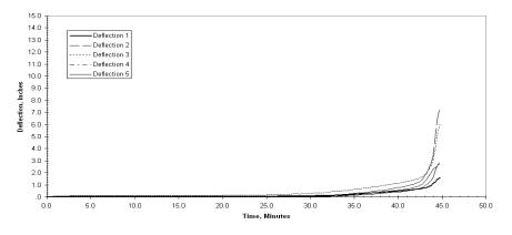
Figure 21 - Plot of Deflections vs. Time for Assembly No. 3
