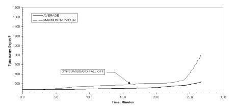
Figure 48 - Plot of Temperature of the Carpet Padding vs. Time for Test Assembly No. 6
