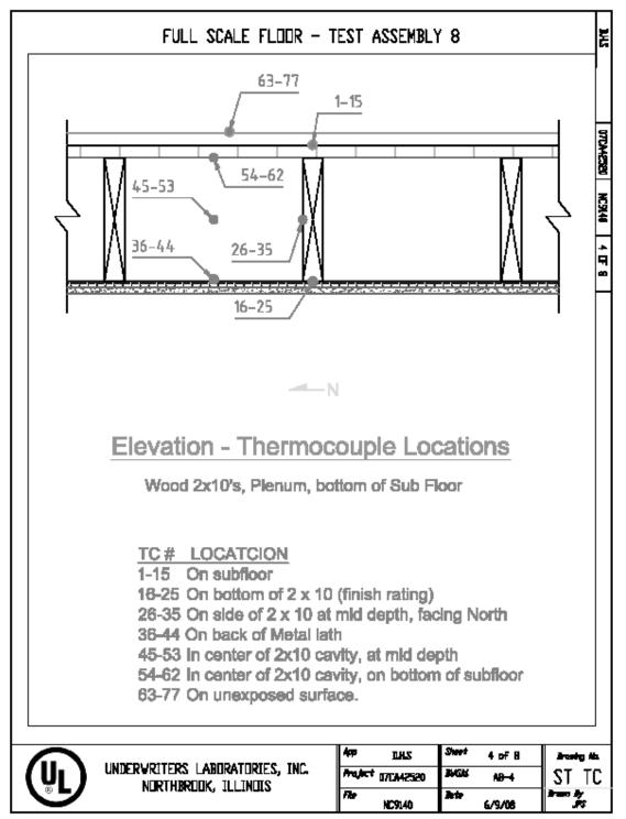
Figure A.8.3 – Thermocouple Locations - Elevation.
