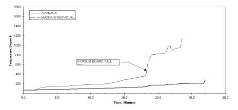
Figure 27 - Plot of Temperature of the Subfloor Temperatures vs. Time
