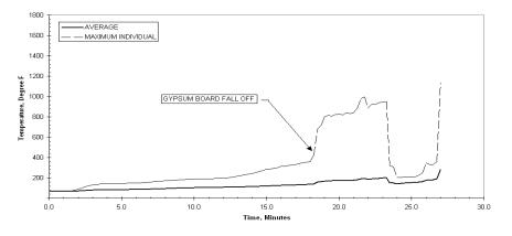
Figure 28 - Plot of Temperature of the Carpet Padding vs. Time for Assembly No. 4
