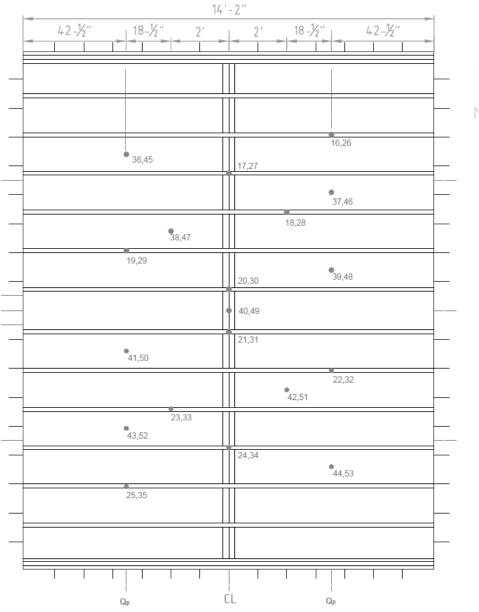
Figure A.1.4 – Thermocouple Locations on Wood Members.
