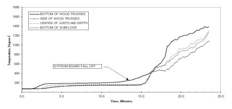
Figure 72 – Plot of Temperature Below Subfloor vs. Time
