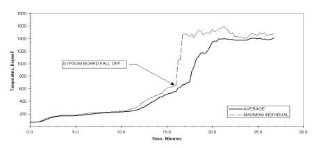
Figure 46 - Plot of Temperature of the Unexposed Surface of Gypsum Board vs. Time for Test Assembly No. 6
