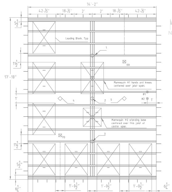
Figure A.1.7 – Loading and Instrumentation Layout (See Figure A.1.8).
