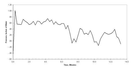
Figure 34 – Furnace Pressure vs. Time for Assembly No. 3
