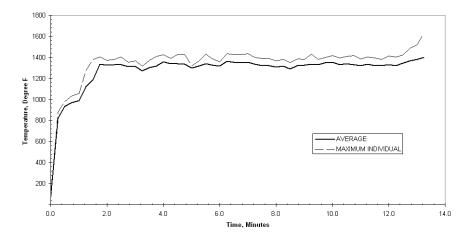
Figure 25 - Plot of Temperatures of Mid Depth Between Wood Trusses vs. Time for Assembly No. 2
