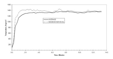
Figure 39 – Plot of Temperatures of the Bottom of the Subfloor between Wood Trusses vs. Time for Assembly No. 3
