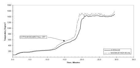
Figure 36 - Plot of Temperature of the Unexposed Surface of Gypsum Board vs. Time for Assembly No. 5
