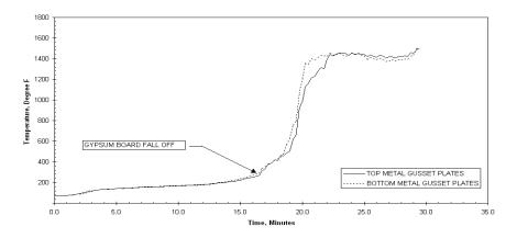
Figure 35 - Plot of Temperature of the Top and Bottom Metal Gusset Plates vs. Time for Assembly No. 5
