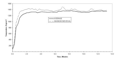
Figure 36 - Plot of Temperatures of Bottom of Wood Trusses vs. Time for Assembly No. 3
