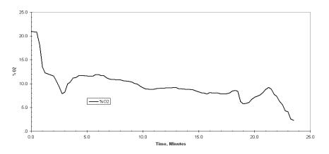
Figure 71 – Oxygen Content vs. Time for Test Assembly No. 9
