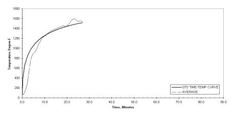
Figure 22 - UL263 Standard Time Temperature Curve and Average Furnace Temperature vs. Time for Assembly No. 4
