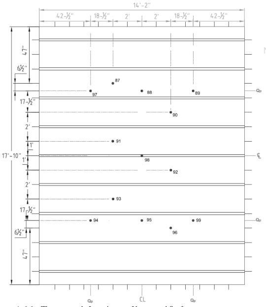
Figure A.6.6 – Thermocouple Locations on Unexposed Surface.
