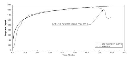
Figure 61 – UL263 Standard Time Temperature Curve and Average Furnace Temperature vs. Time for Test Assembly No. 8
