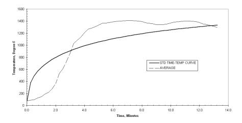
Figure 20 - UL263 (ASTM E119) Standard Time Temperature Curve and Average Furnace Temperature vs. Time for Assembly No. 2
