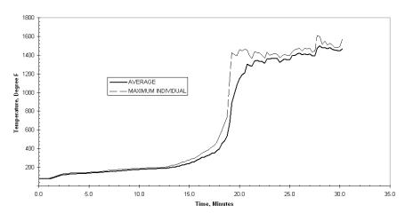
Figure 4 - Plot of Temperature of the Average and Maximum Individual Side Of Wood Trusses vs. Time for Assembly No. 1
