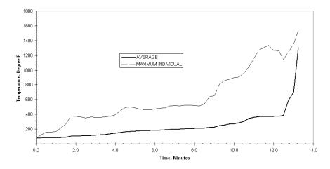
Figure 29 - Plot of Temperatures of Top of Subfloor vs. Time for Assembly No. 2
