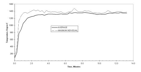
Figure 37 – Plot of Temperatures of Side of Wood Trusses vs. Time for Assembly No. 3
