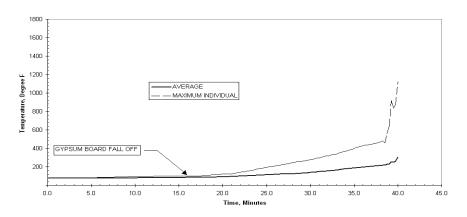
Figure 57 – Plot of Temperature of the Roofing Felt vs. Time for Test Assembly No. 7
