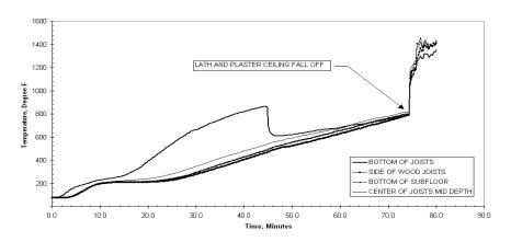
Figure 64 - Plot of Temperatures Below Subfloor vs. Time for Test Assembly No. 8
