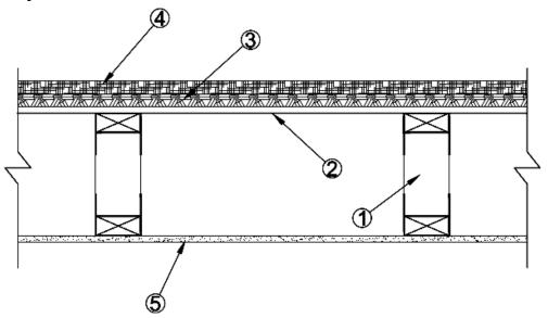
1) 14 in. wood truss with metal gussets spaced 24 in. O.C. supplied with bottom chord splices with strongback.
