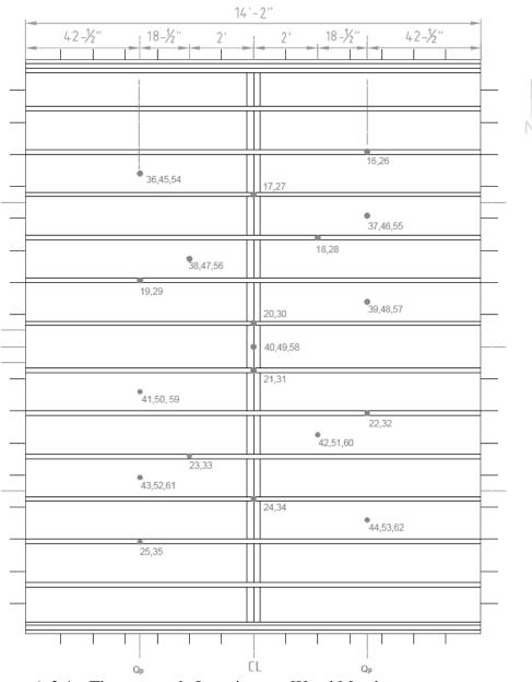
Figure A.3.4 – Thermocouple Locations on Wood Member.
