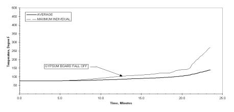
Figure 75 – Plot of Temperatures of the Unexposed Surface vs. Time
