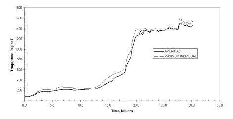
Figure 15 - Plot of Temperatures over the Flexible Duct at Center Span vs. Time for Assembly No. 1
