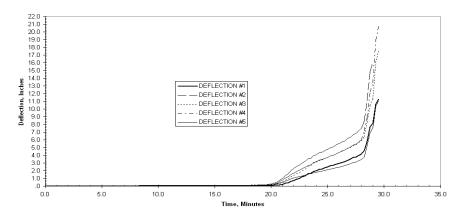
Figure 40 - Plot of Deflections vs. Time for Assembly No. 5
