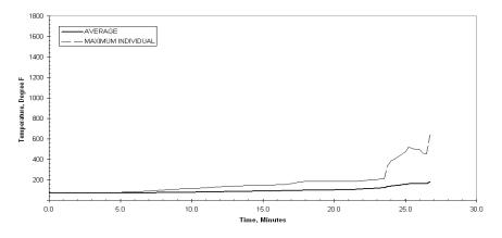
Figure 49 - Plot of Temperatures of the Unexposed Surface vs. Time for Test Assembly No. 6
