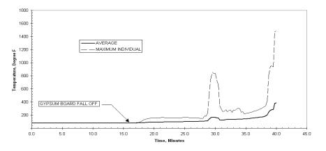
Figure 58 - Plot of Temperatures of the Unexposed Surface vs. Time for Test Assembly No. 7
