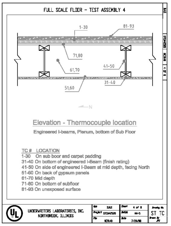
Figure A.4.3 – Thermocouple Locations - Elevation.
