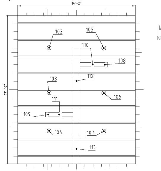
102 - 107 - On top of can lights over can light venting 108 - 109 - On top fo flexible duct right before junction of supply register inlet. 110 - 111 - On top of flexible duct at mid span
