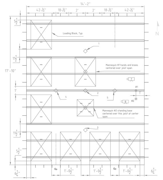
Figure A.6.7 – Loading and Instrumentation Layout (See Figure A.6.8)
