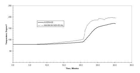
Figure 12 - Plot of Temperatures of the Unexposed Surface vs. Time for Assembly No. 1
