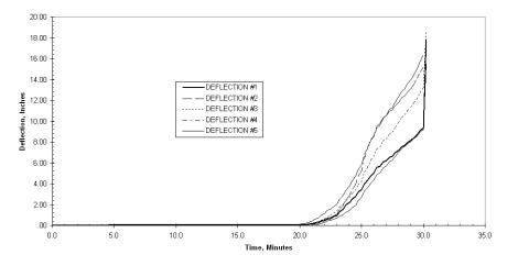
Figure 19 - Plot of Deflections vs. Time for Assembly No. 1
