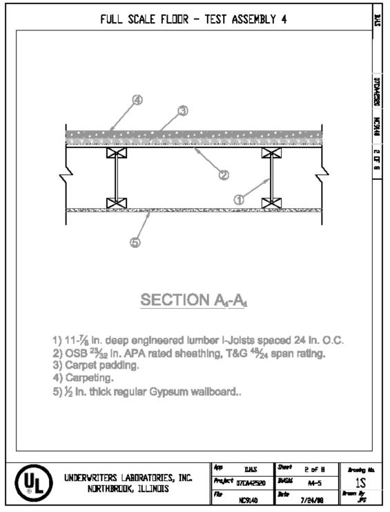
Figure A.4.2 – Construction Layout Section A<sub>4</sub>-A<sub>4</sub>.
