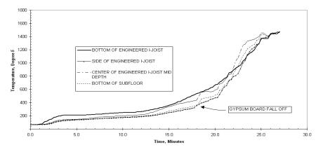
Figure 25 - Plot of Temperatures Below Subfloor vs. Time for Assembly No. 4
