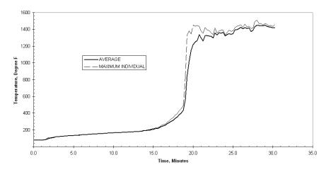
Figure 7 - Plot of Temperature of the Bottom Metal Gusset Plates vs. Time for Assembly No. 1
