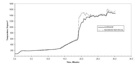
Figure 18 - Plot of Temperatures of the Truss Splice 2 in. from Metal Gussets vs. Time for Assembly No. 1
