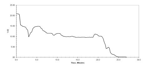
Figure 24 - Oxygen Content vs. Time for Assembly No. 4
