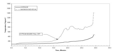
Figure 37 - Plot of Temperature of the Subfloor Temperatures vs. Time for Assembly No. 5
