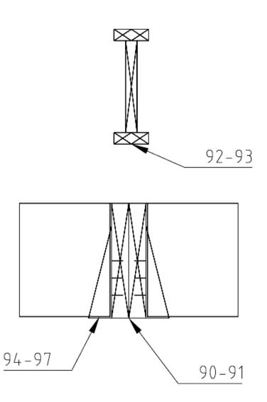
Figure A.3.8 – Elevation of Thermocouple Locations on LVL Assembly and Metal Connectors.
