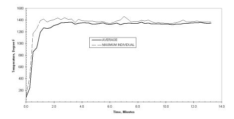
Figure 45 – Plot of Temperatures of the LVL Assembly and Metal Connectors vs. Time
