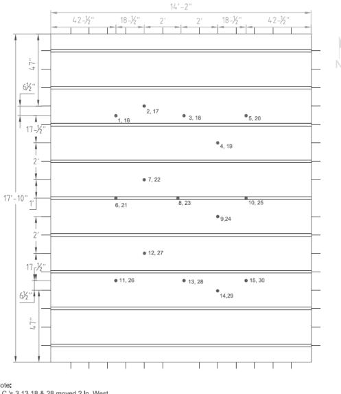
Note: T.C.'s 3,13,18 & 28 moved 2 In. West. T.C.'s 8,23 moved 2 in. East Due to sheathing Being Cut short from
