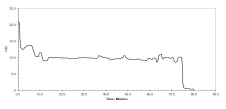
Figure 63 – Oxygen Content vs. Time for Test Assembly No. 8
