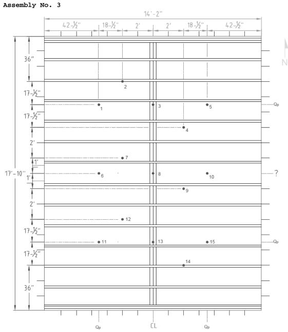
Figure A.3.5 – Thermocouple Locations on Subfloor.
