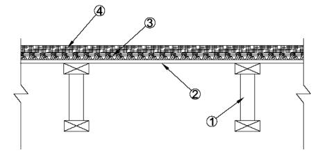
1) 14 in. Deep wood truss with glued finger joints spaced 24 in. O.C.
