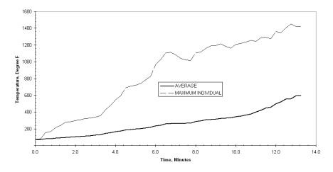
Figure 42 – Plot of Temperatures of the Top of the Subfloor vs. Time for Assembly No. 3
