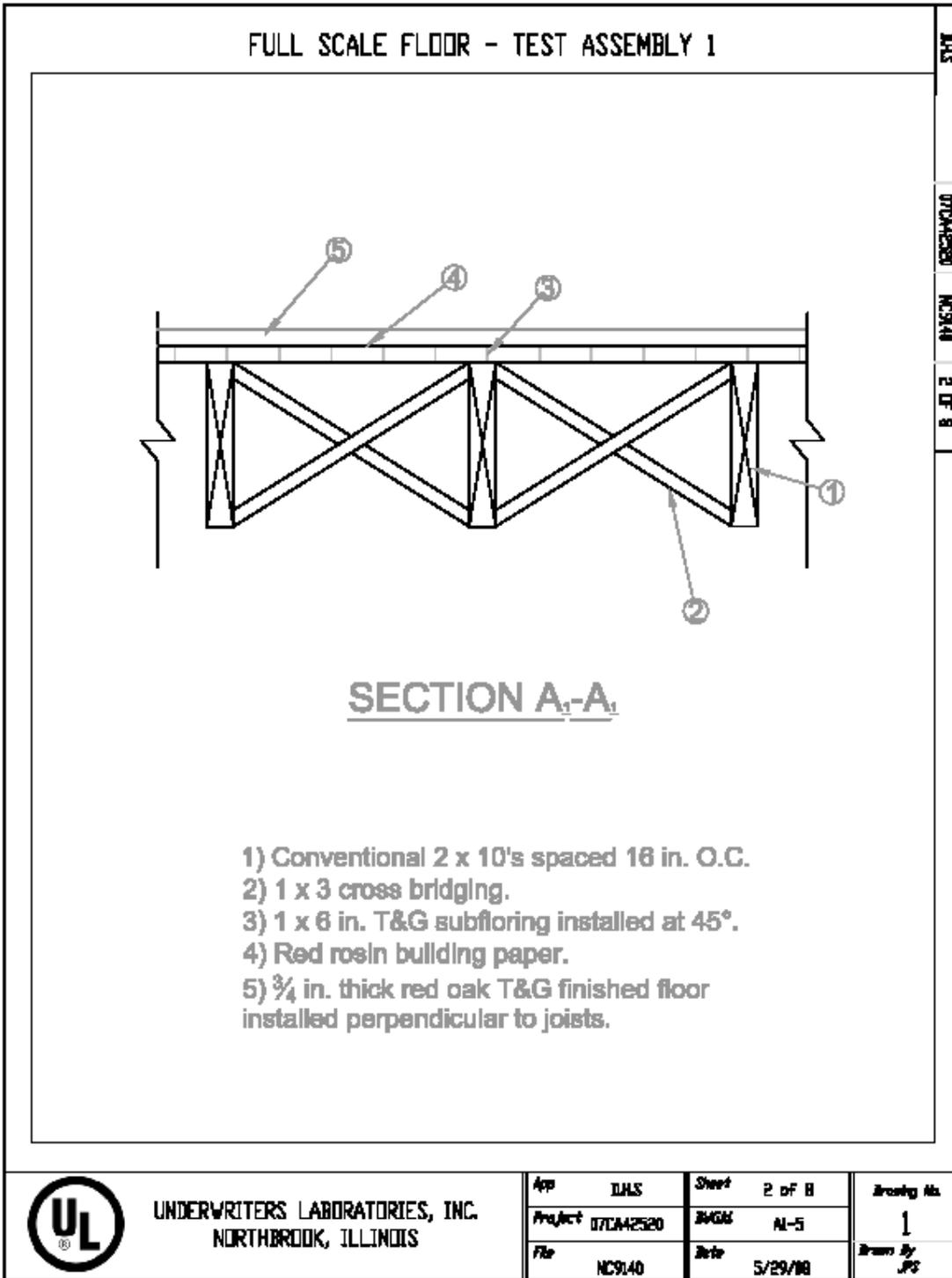
Figure A.1.2 – Construction Layout Section A<sub>1</sub>-A<sub>1</sub>.
