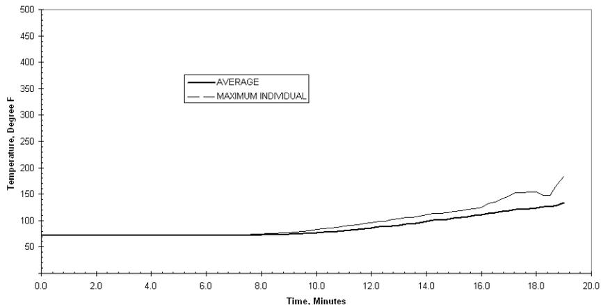
**Figure 4 - Plot of the Unexposed Surface Temperatures vs. Time for Assembly No. 1**
