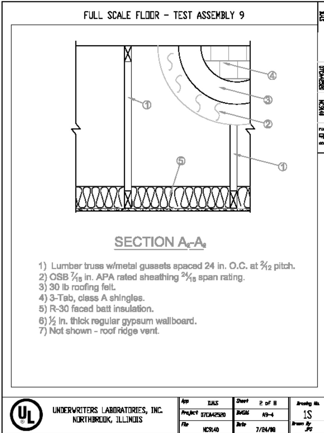
Figure A.9.2 – Construction Layout Section A<sub>9</sub>-A<sub>9</sub>.
