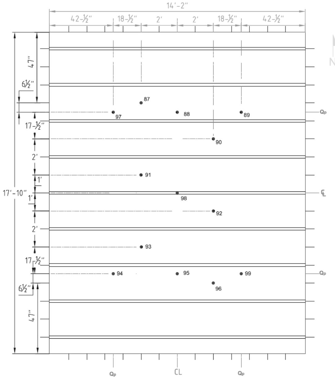
Figure A.6.6 – Thermocouple Locations on Unexposed Surface.
