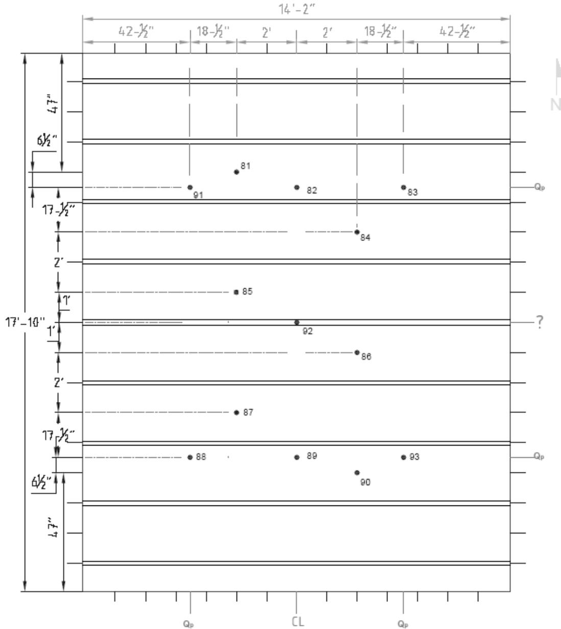
Figure A.4.6 – Thermocouple Locations on Unexposed Surface.
