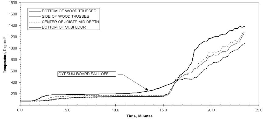
Figure 72 – Plot of Temperature Below Subfloor vs. Time
