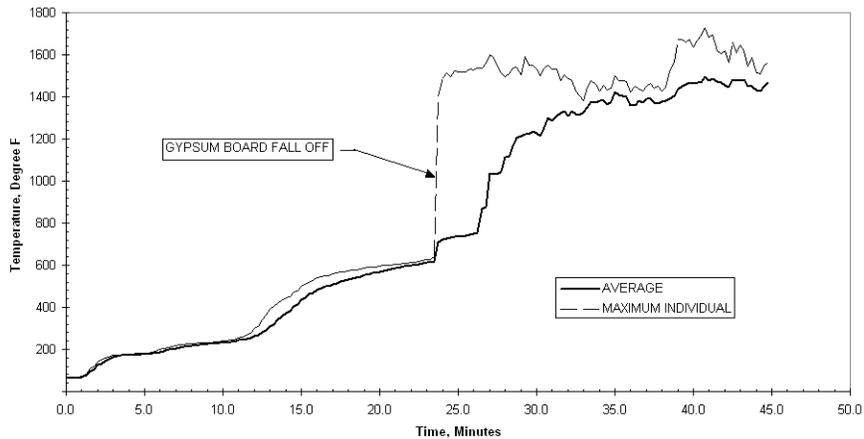
**Figure 18 - Plot of Temperature of the Unexposed Surface of Gypsum Board vs. Time for Assembly No. 3**
