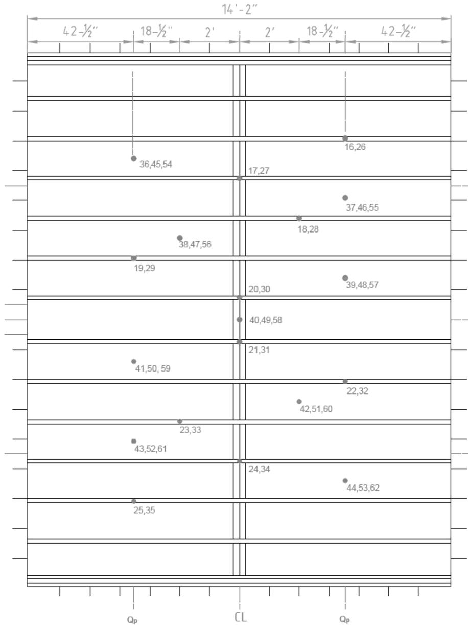
Figure A.3.4 – Thermocouple Locations on Wood Member.
