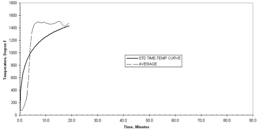
**Figure 1 - UL263 Standard Time Temperature Curve and Average Furnace Temperature vs. Time for Assembly No. 1**
