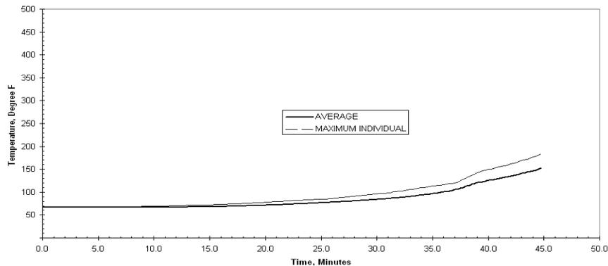
**Figure 20 - Plot of Temperatures of the Unexposed Surface vs. Time for Assembly No. 3**
