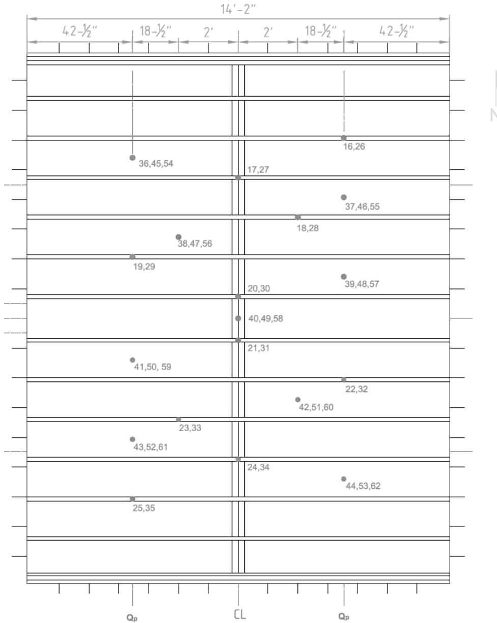
Figure A.8.4 – Thermocouple Locations on Wood Members.
