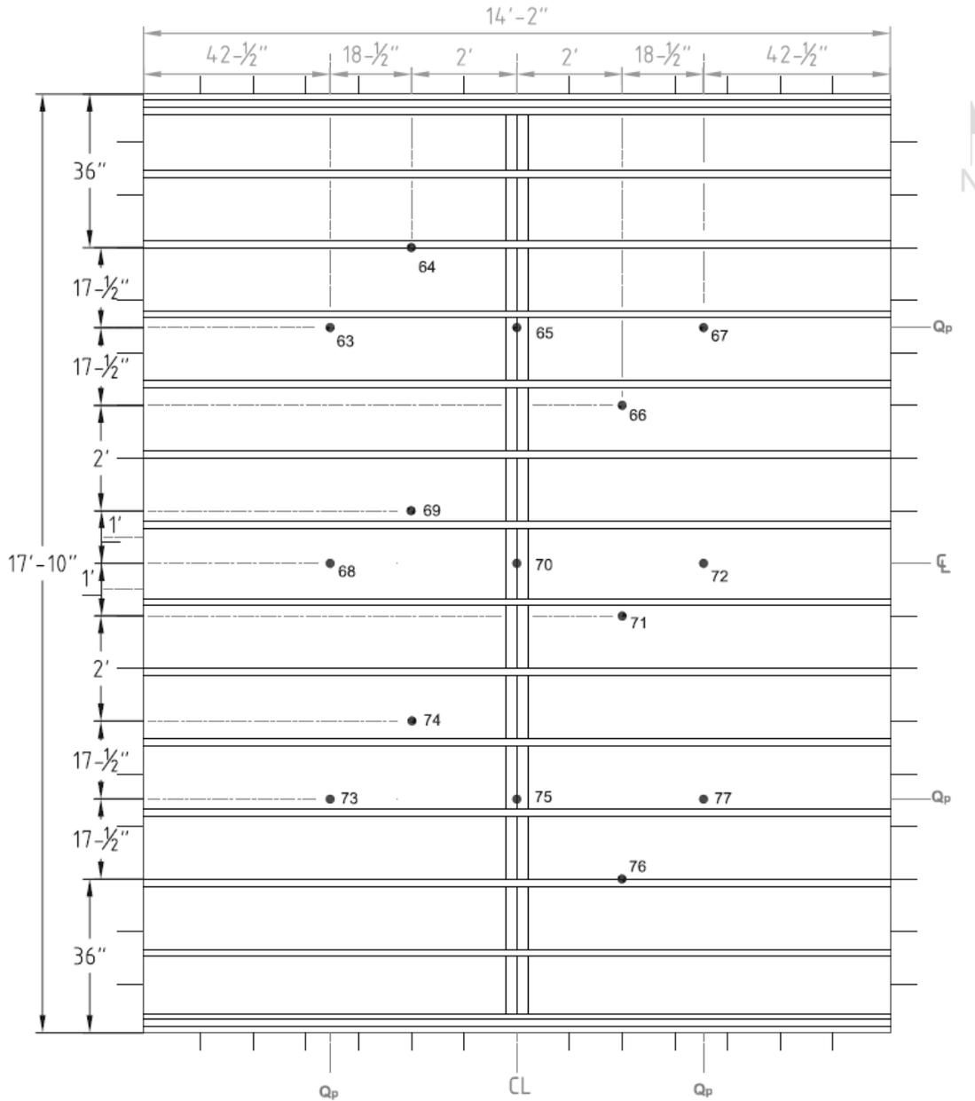
Figure A.8.6 – Thermocouple Locations on Unexposed Surface.
