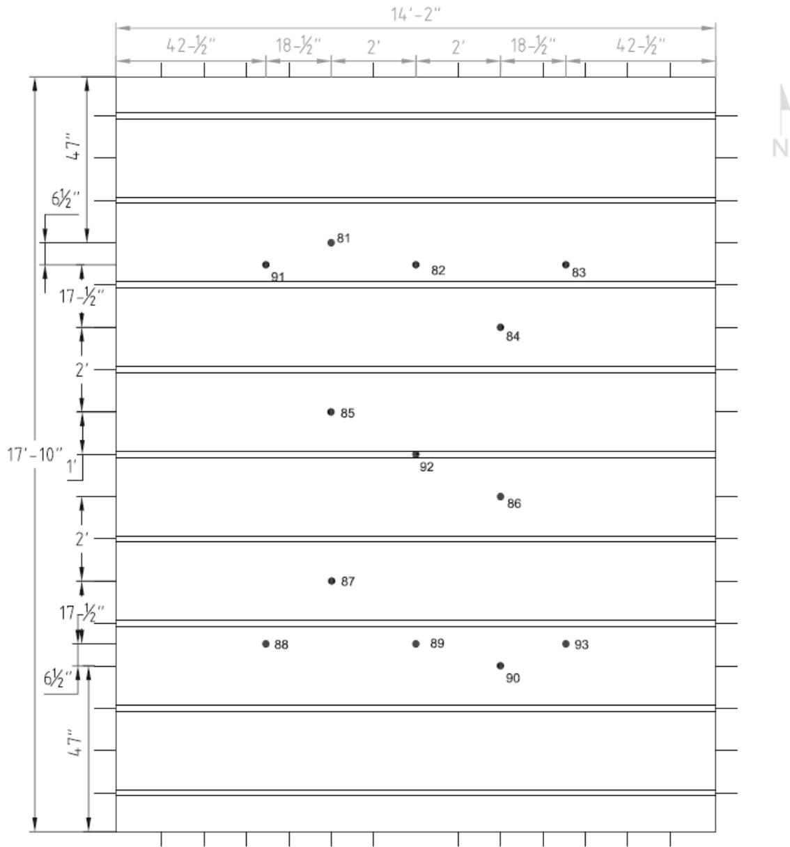
Figure A.9.6 – Thermocouple Locations on Unexposed Surface.
