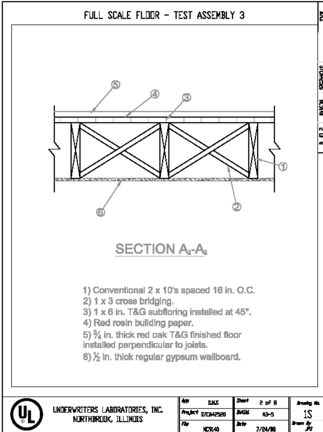
Figure A.3.2 – Construction Layout Section A<sub>3</sub>-A<sub>3</sub>.
