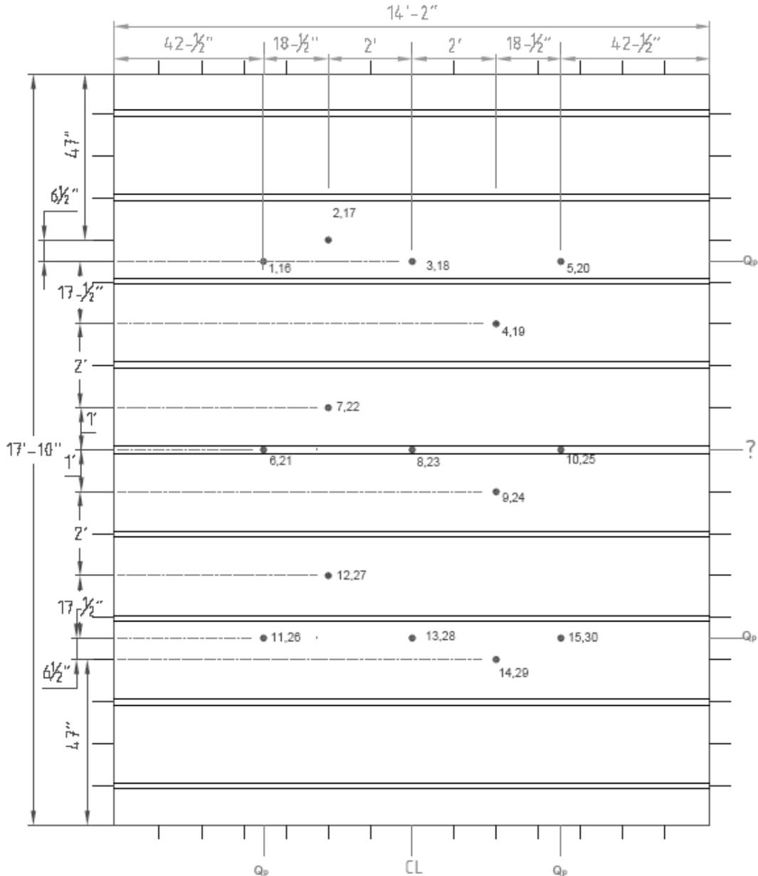
Figure A.4.5 – Thermocouple Locations on Subfloor and Carpet Padding.
