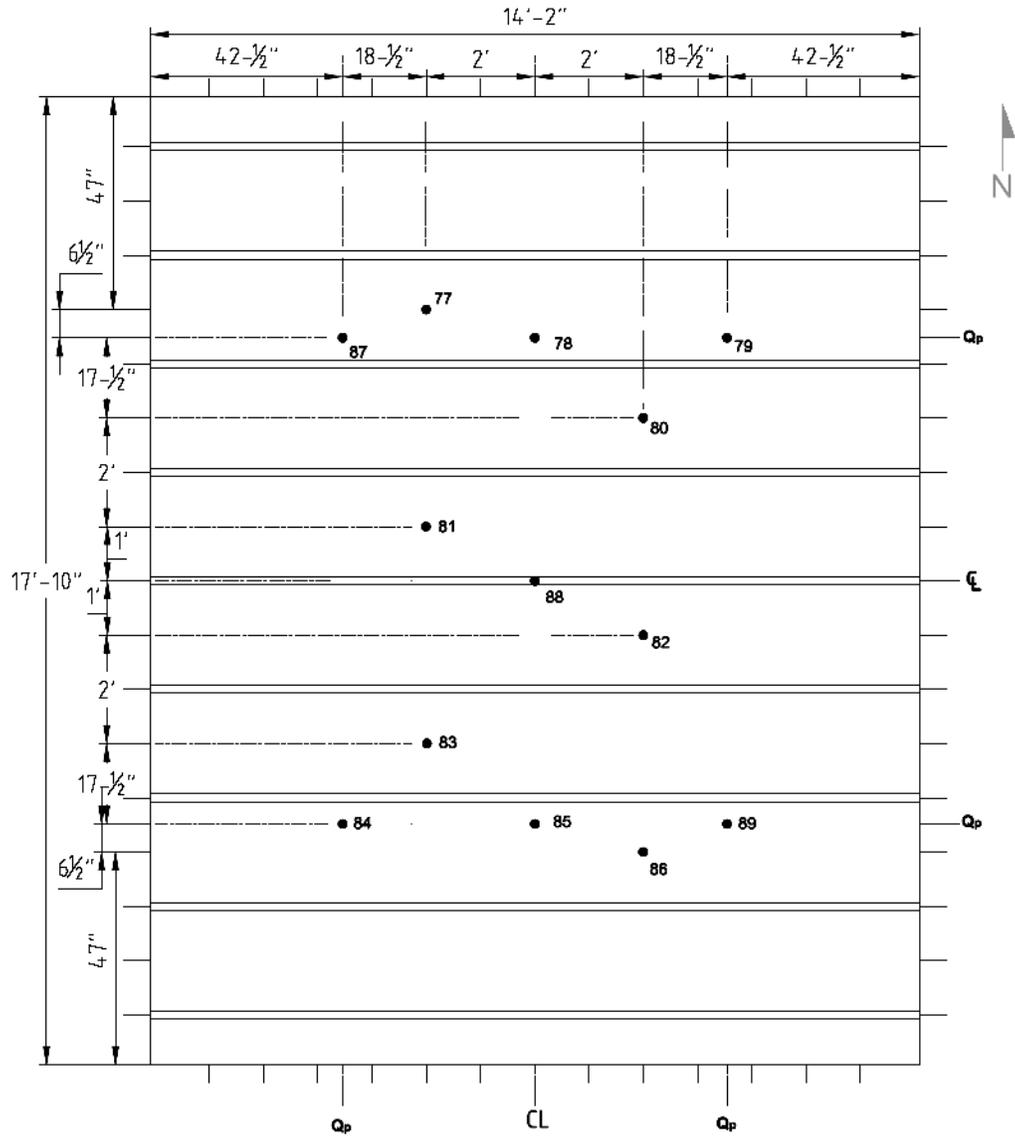
Figure A.2.6 – Thermocouple Locations on Unexposed Surface.
