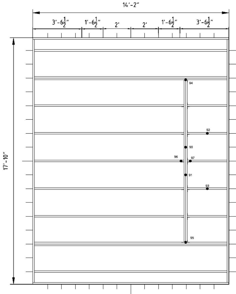
**Mis Structural Thermocouple Locations**
