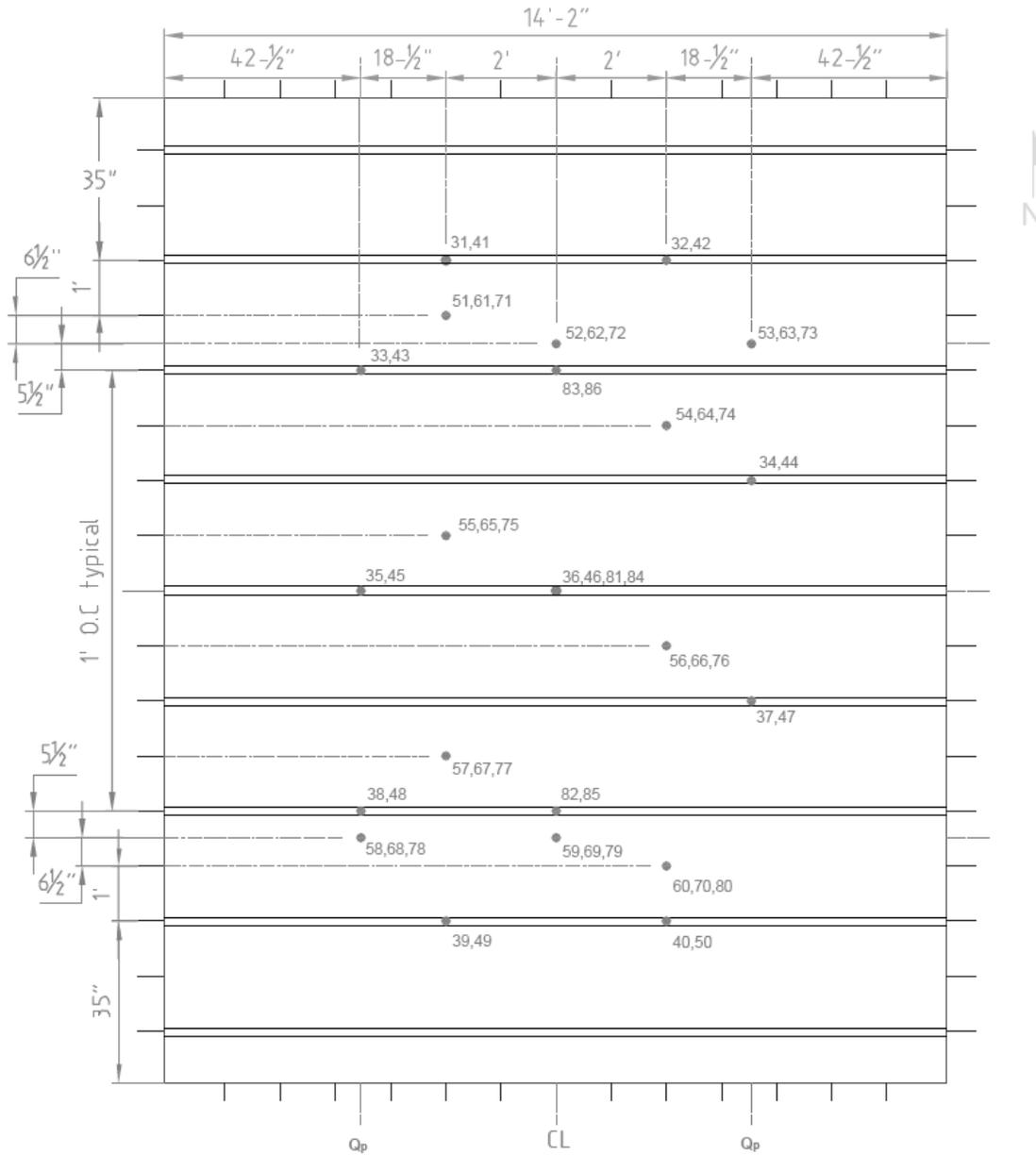
Figure A.5.4 – Thermocouple Locations on Wood Members.
