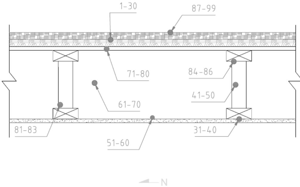
**Elevation - Thermocouple Locations**
