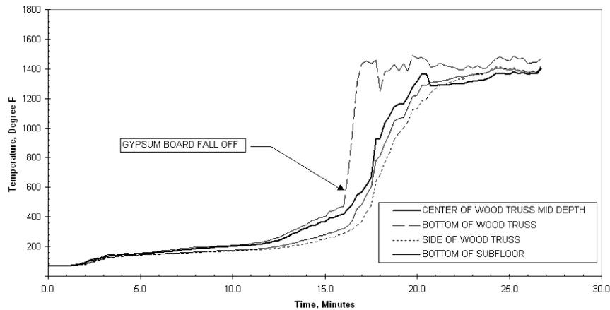
**Figure 44 - Plot of Temperatures of Below Subfloor vs. Time**
