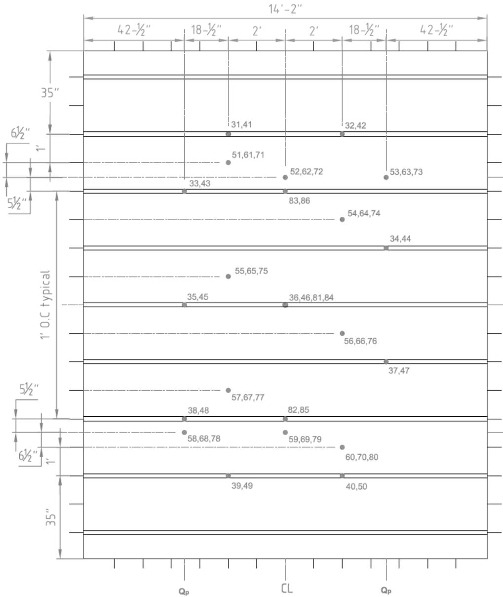
Figure A.6.4 – Thermocouple Locations on Wood Members.
