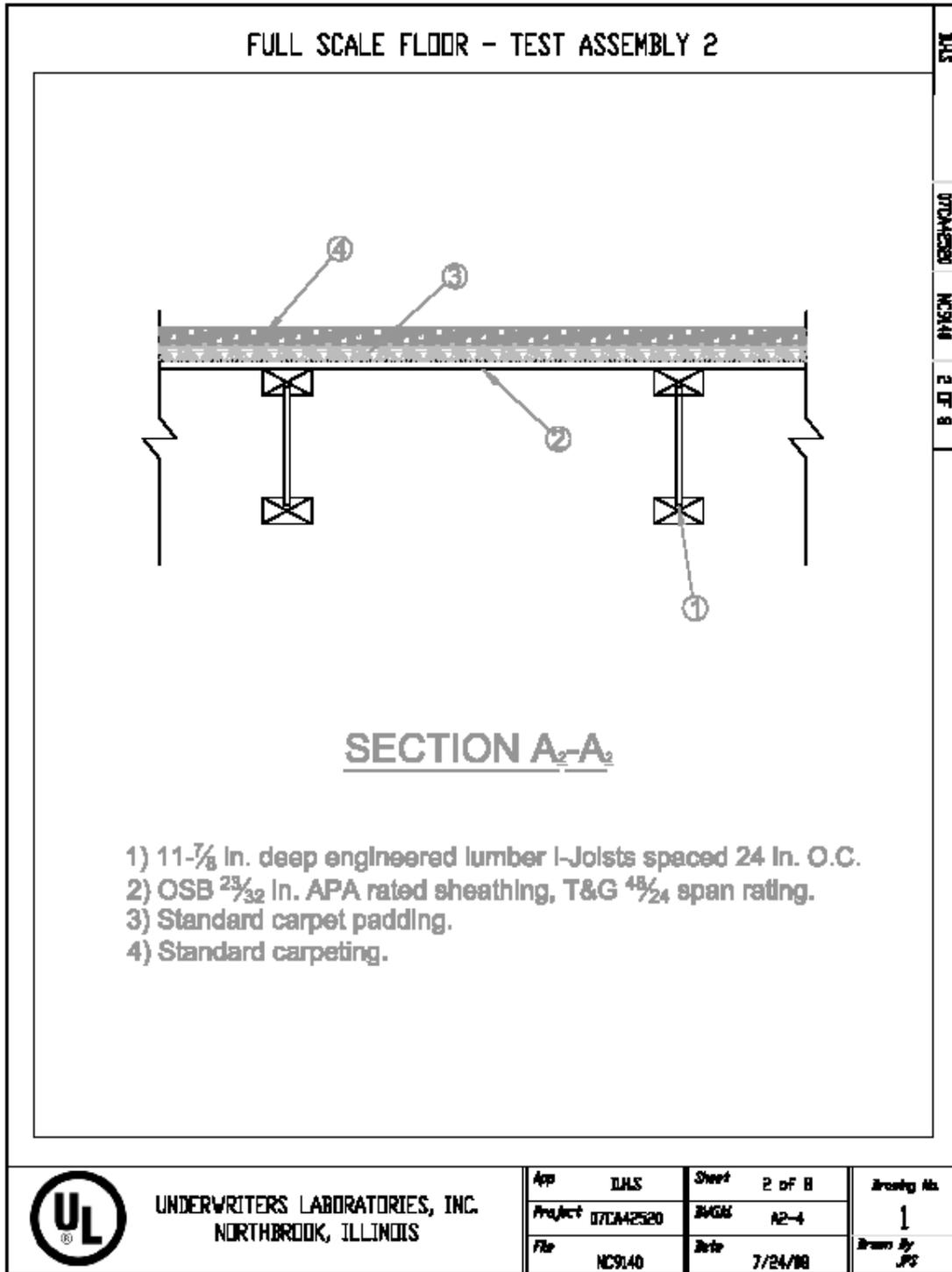
Figure A.2.2 – Construction Layout Section A<sub>2</sub>-A<sub>2</sub>.
