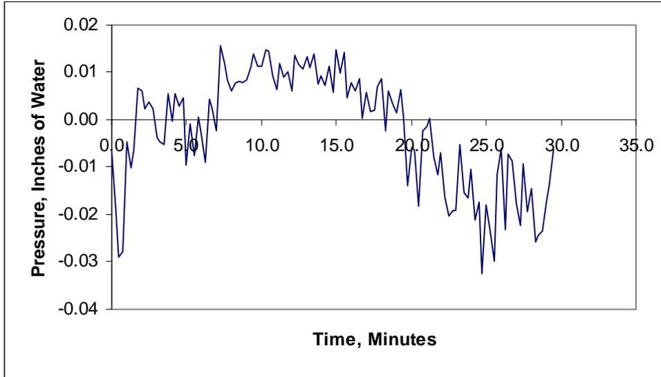
**Figure 32 - Furnace Pressure vs. Time for Assembly No. 5**
