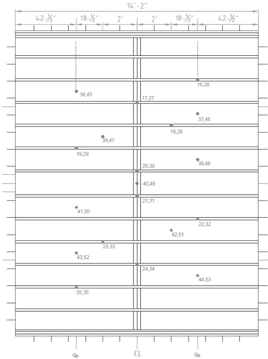
Figure A.1.4 – Thermocouple Locations on Wood Members.
