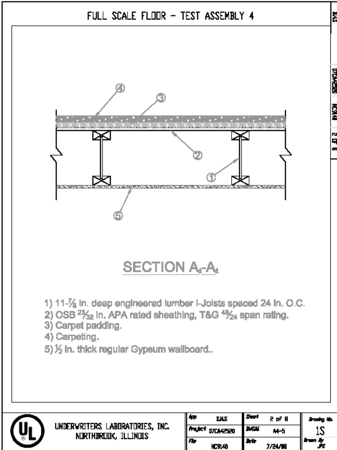
Figure A.4.2 – Construction Layout Section A<sub>4</sub>-A<sub>4</sub>.
