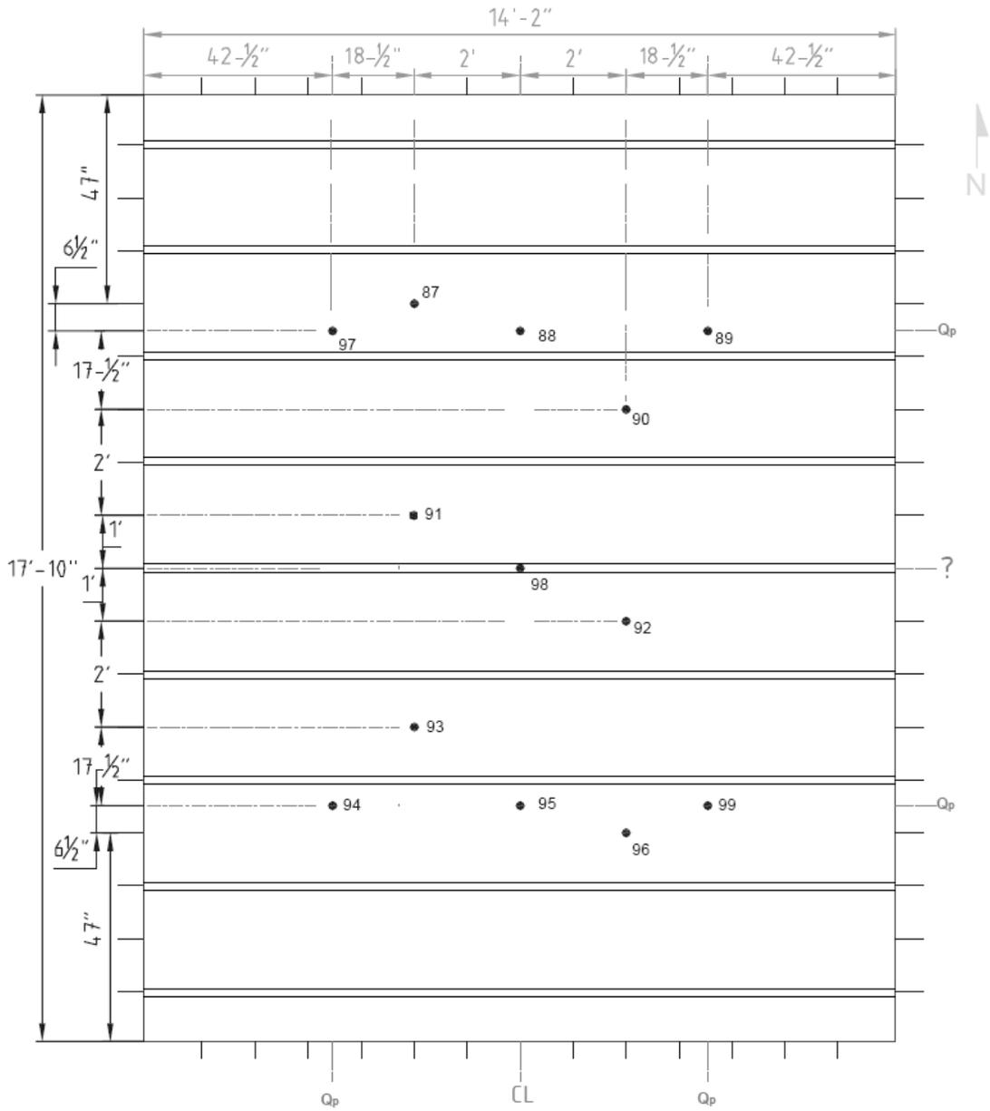
Figure A.5.6 – Thermocouple Locations on Unexposed Surface.
