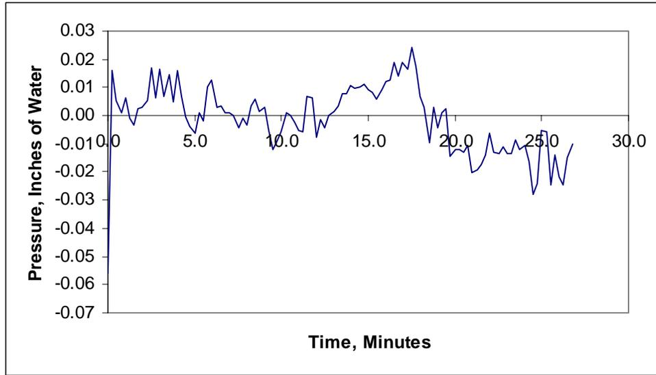
Figure 42 - Furnace Pressure vs. Time for Assembly No. 6
