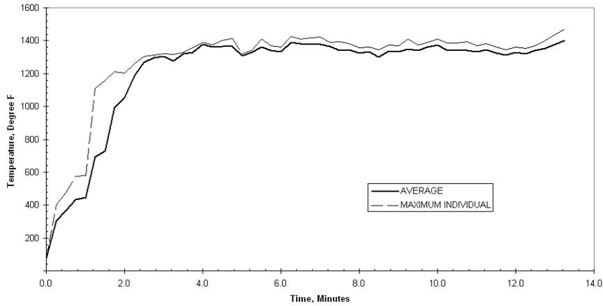
**Figure 27 - Plot of Temperatures of Top Glued Finger Joints vs. Time for Assembly No. 2**
