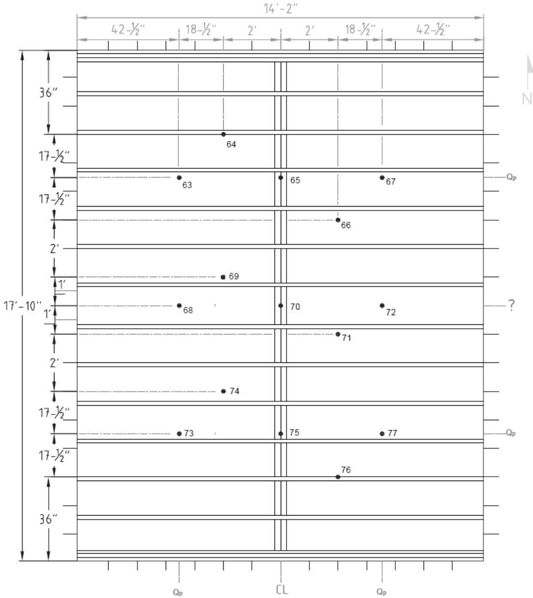
Figure A.3.6 – Thermocouple Locations on Unexposed Surface.
