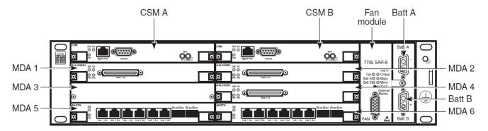
Figure 1-1: Front View of the Alcatel Lucent 7705 MPLS Router, Showing Redundant Control and Switching Modules
