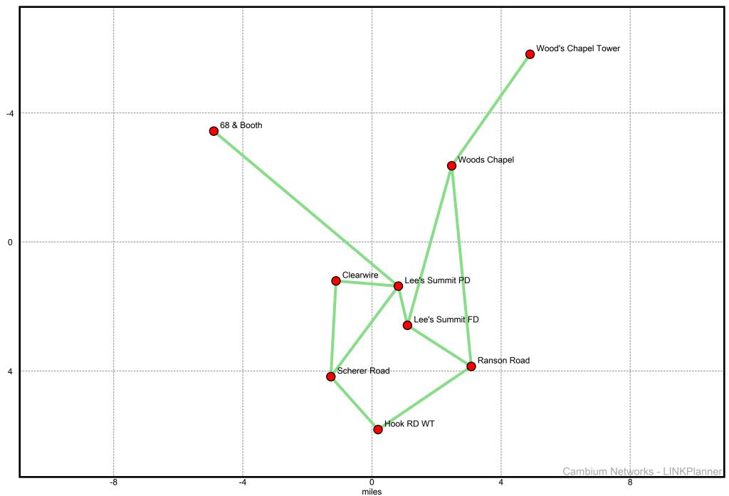
Each Lee's Summit site has a Nokia 7705 MPLS router with dual routing engine for redundancy. One Nokia 7705 MPLS router will be positioned at the Wood's Chapel MARRS site connecting into Lee's Summit microwave ring. The Nokia 7705 routers utilizing MPLS were chosen to stay in line with the MARRS regional plan to convert the circuit based network to an MPLS Ethernet backhaul throughout the regional system.
