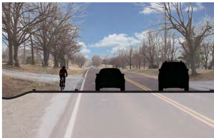
Figure 9. Cross section illustrating road widening of Smart Road to accommodate cyclists.
