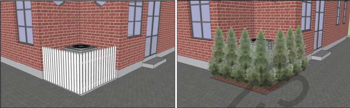
**HVAC units and condensers at rear facades shall be screened through fencing or landscaping. Units should have 36 inches of clearance to allow for maintenance and servicing.**
