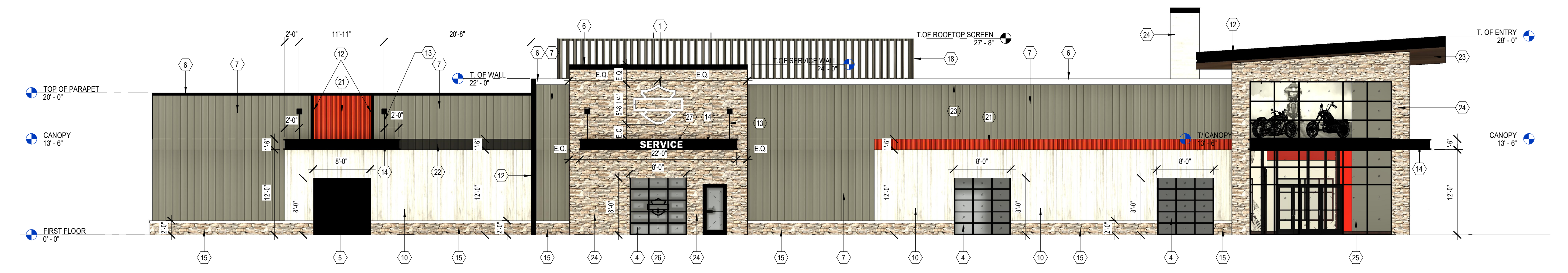
4 WEST ELEVATION SCALE: 1/8" = 1'-0" METAL PANELS: 1,445 S.F. (36%) FAUX FIBER CEMENT: 1,510 S.F. (38%) THIN STONE VENEER: 375 S.F. (10%) WINDOWS/DOORS: 650 S.F. (16%) FACADE TOTAL: 3,980 S.F. (100%)
