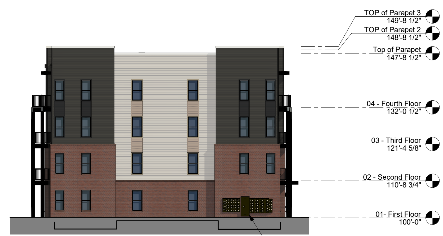
3 BLDG C-Right Elevation-C scale: 1/16" = 1'-0"
