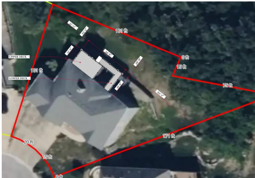
Figure 4 - Plot plan showing proposed replacement deck and catwalk shaded in red. Stairs shown with hatching.
