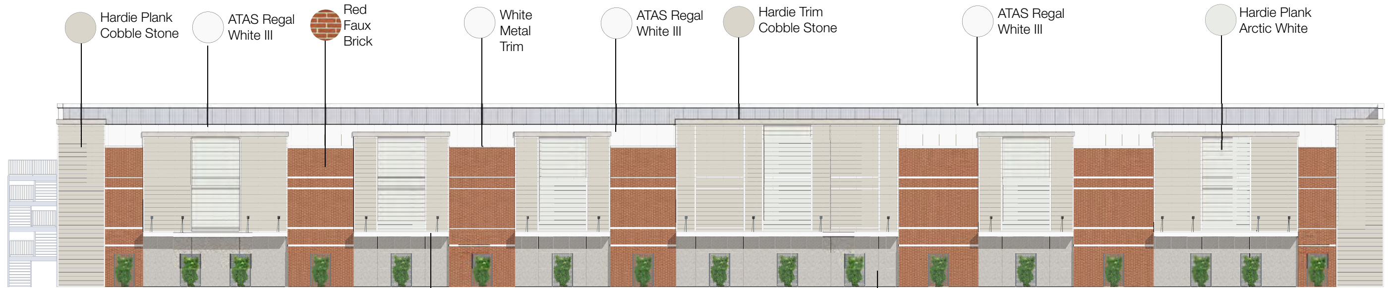
NORTH ELEVATION - BLDG. A
