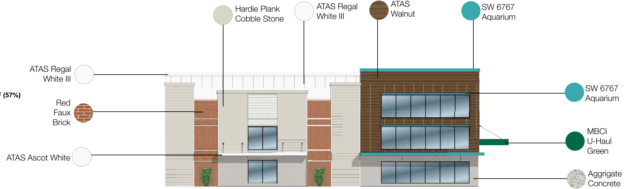
WEST ELEVATION - BLDG. A
