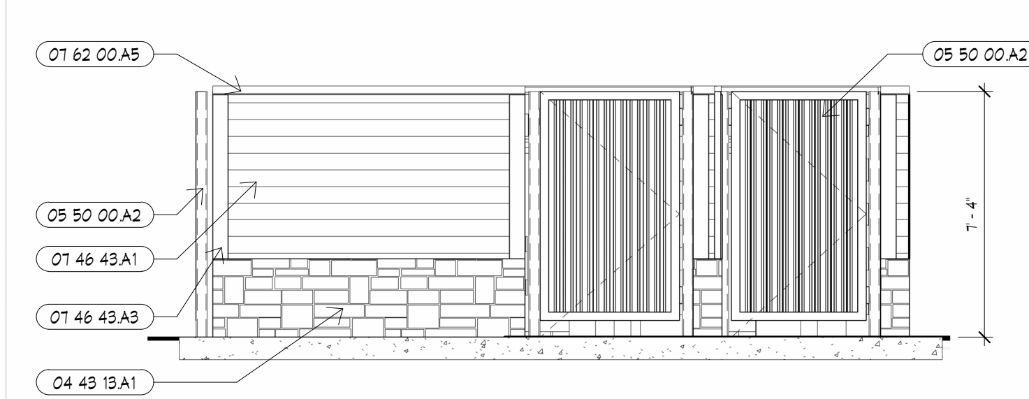
A3 SITE - TRASH ENCLOSURE SIDE 1/4" = 1'-0"
