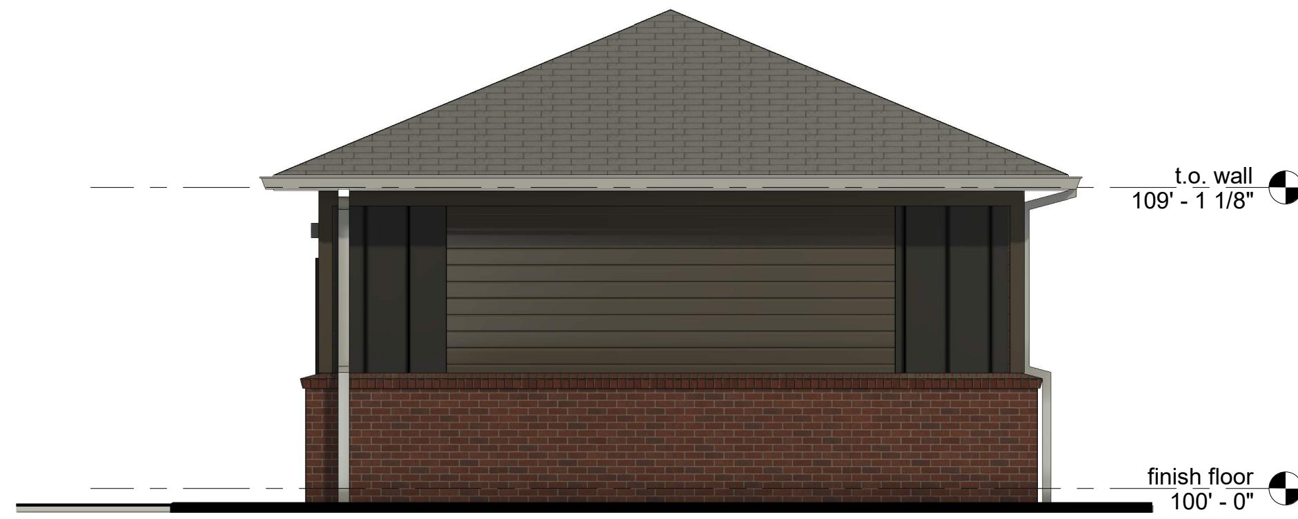
3 West Elevation scale: 1/4" = 1'-0" Elevation Faces Parking
