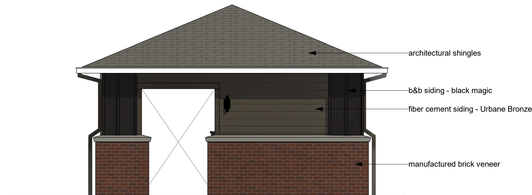
4 Left Elevation scale: 1/4" = 1'-0" Elevation Faces Parking
