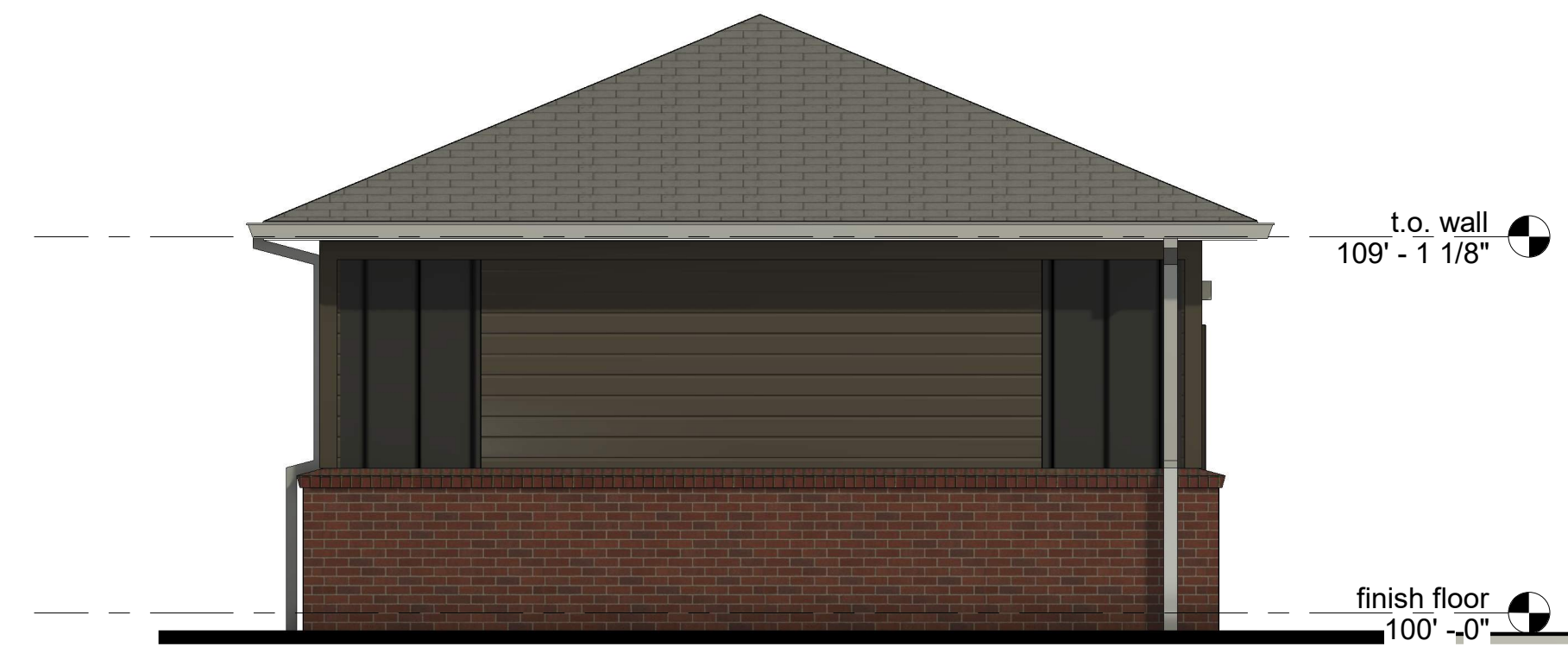
1 East Elevation scale: 1/4" = 1'-0" Elevation Faces Parking
