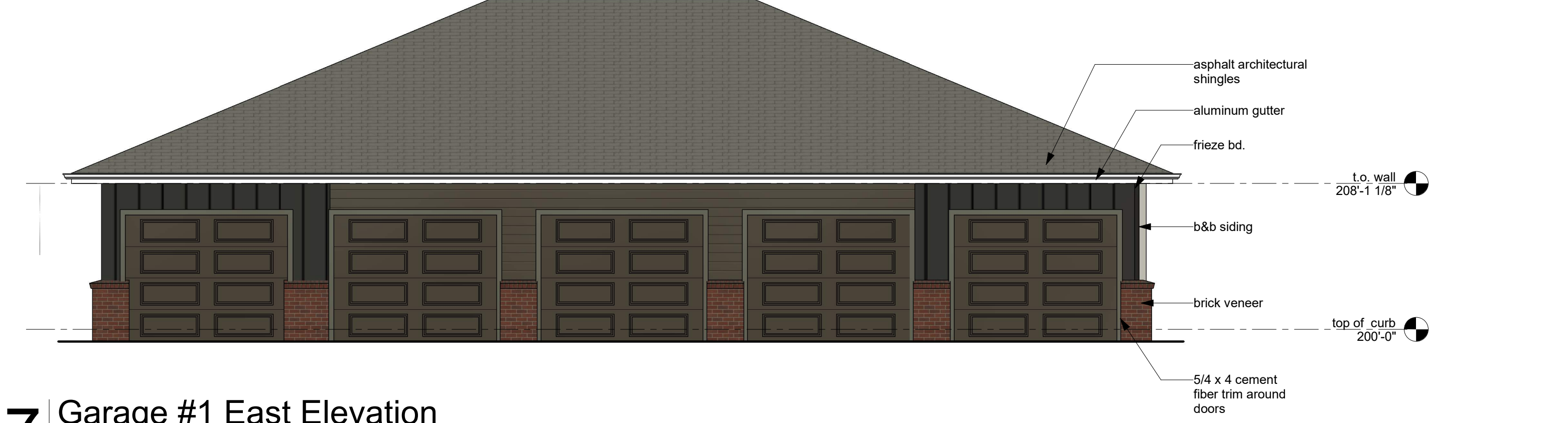
7 Garage #1 East Elevation scale: 3/16" = 1'-0" Elevation Faces Parking
