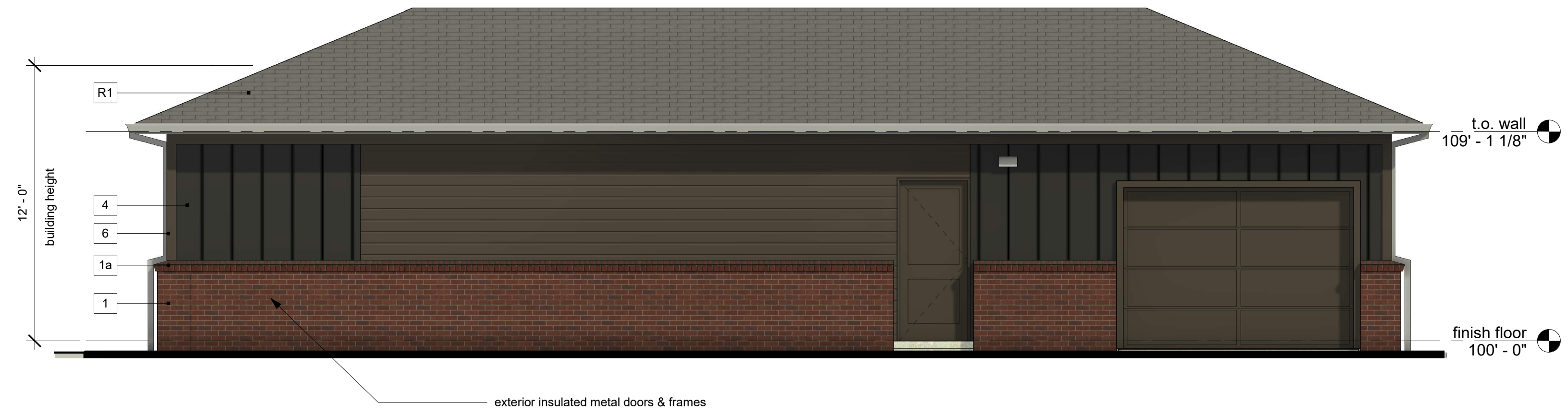
2 North Elevation scale: 1/4" = 1'-0" Elevation Faces Parking
