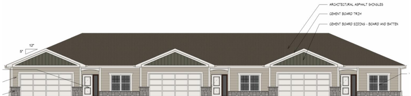
Figure 4 - Front elevation (villas).
