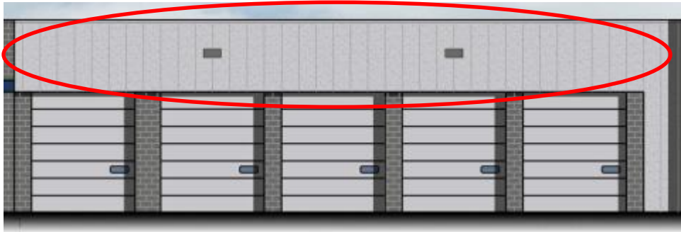
Figure 2 – Stucco-finished metal wall panel (south elevation)
