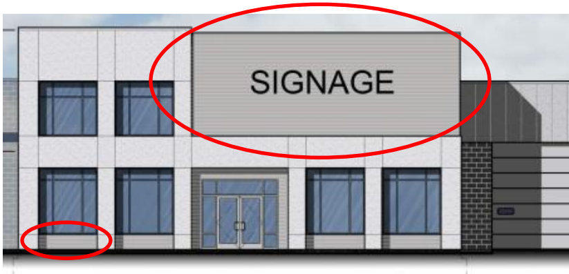
Figure 1 - Architectural ribbed metal (east elevation)
