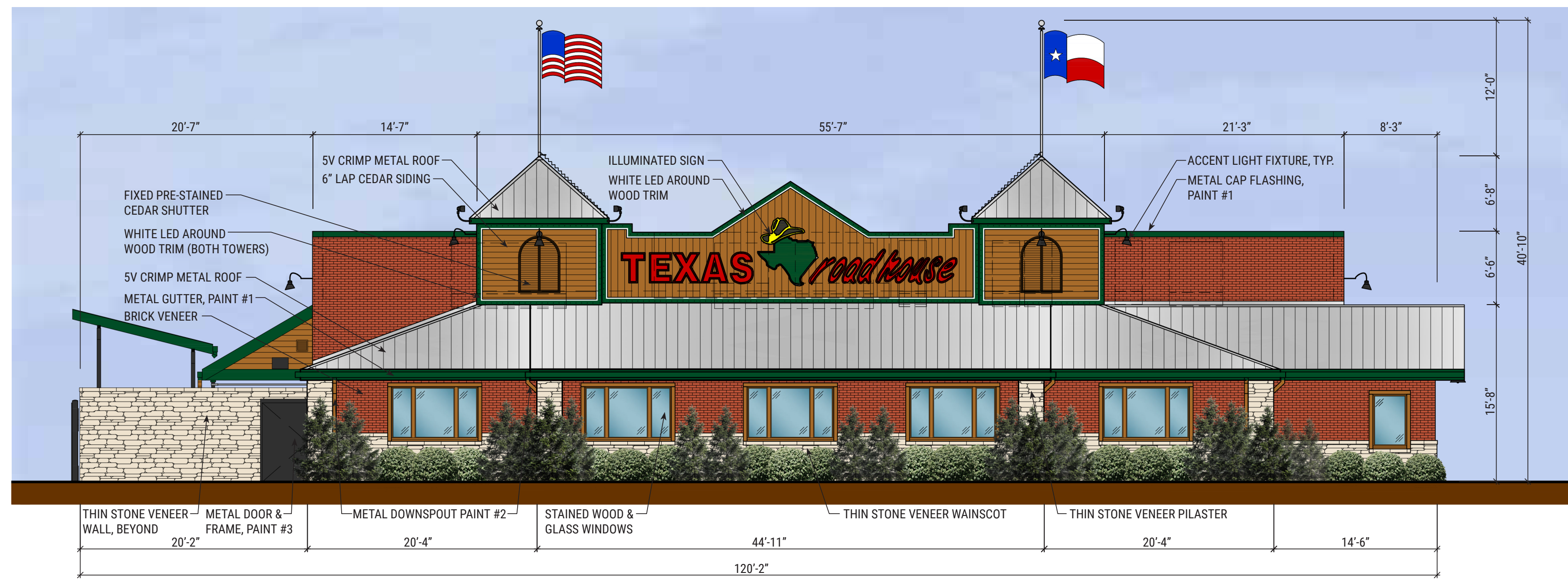
FRONT ELEVATION (WEST)
