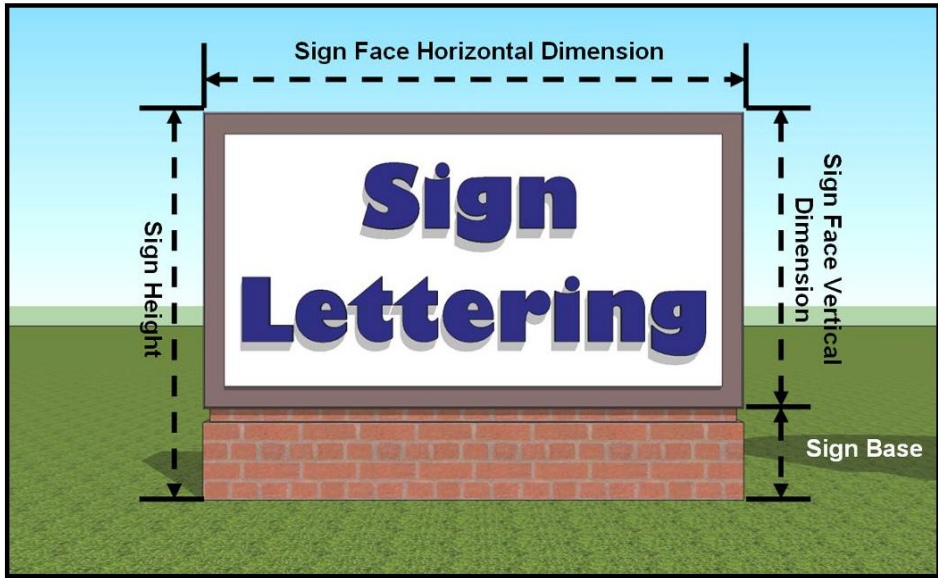
Measuring Sign Face Area and Sign Height
