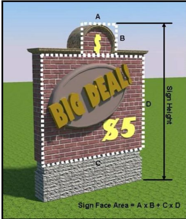
Measuring Sign Face and Sign Height
