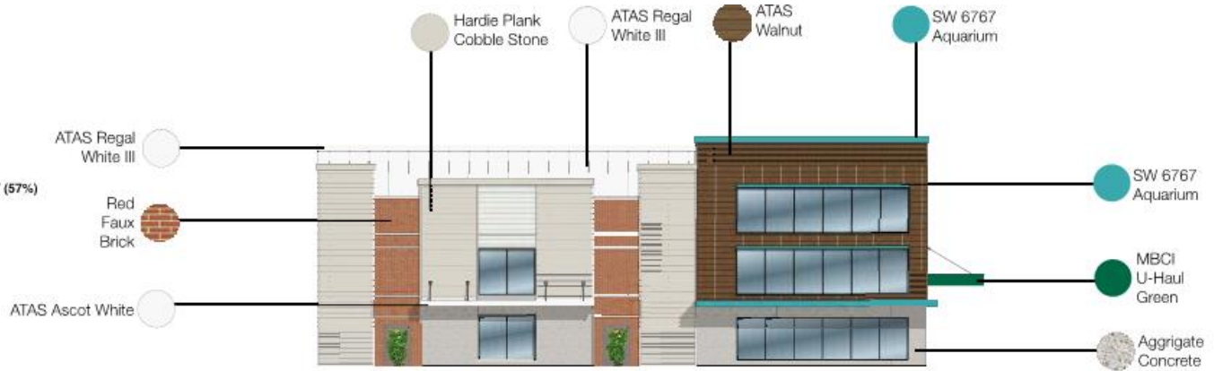
WEST ELEVATION - BLDG. A
