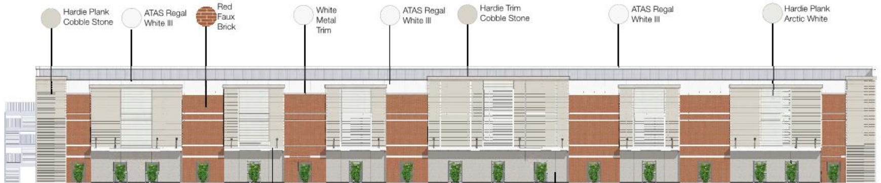
NORTH ELEVATION - BLDG. A
