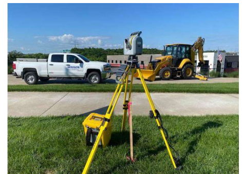
Trimble SX 10 set up for a bridge survey terrestrial lidar scanning.
