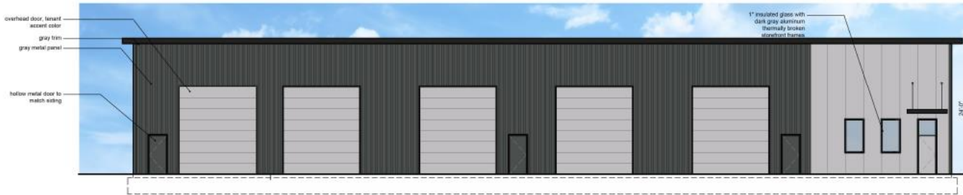
1 West Elevation - Lot B Building scale: 1/8" = 1'-0"
