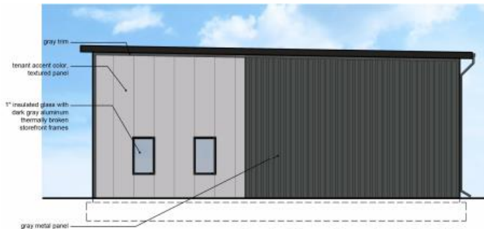
2 South Elevation - Lot B Building scale: 1/8" = 1'-0"
