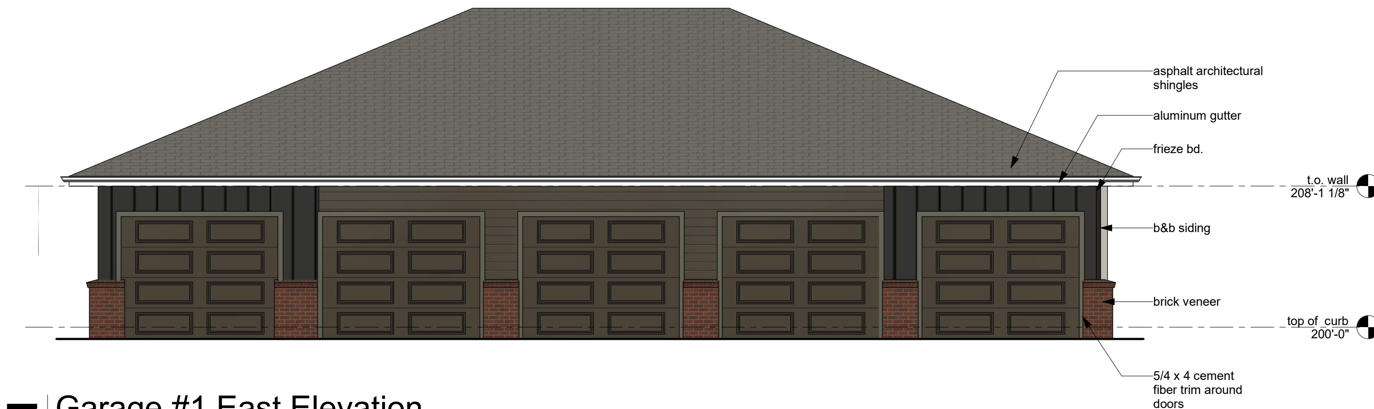
7 Garage #1 East Elevation scale: 3/16" = 1'-0" Elevation Faces Parking
