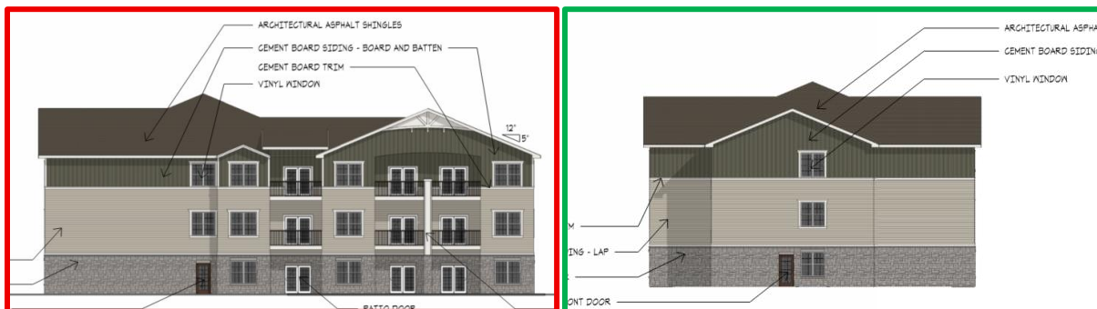
Figure 7 - Comparison of original end of the independent living wing facing Ridgewood Hills to the north (left image outlined in red) and revised building elevation of the end of the independent living wing facing Ridgewood Hills to the north (right image outlined in green).
