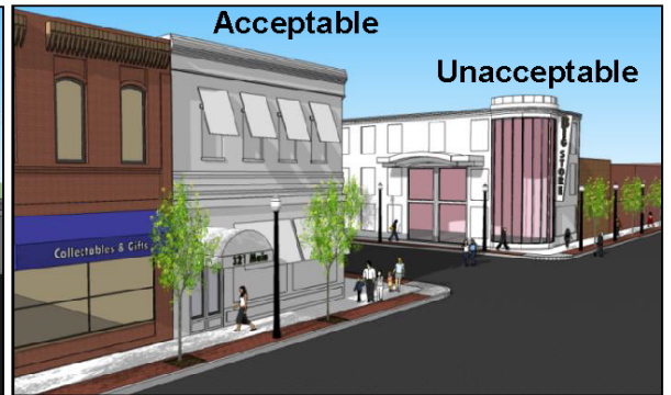
Examples of buildings that do and do not contribute to human scale.
