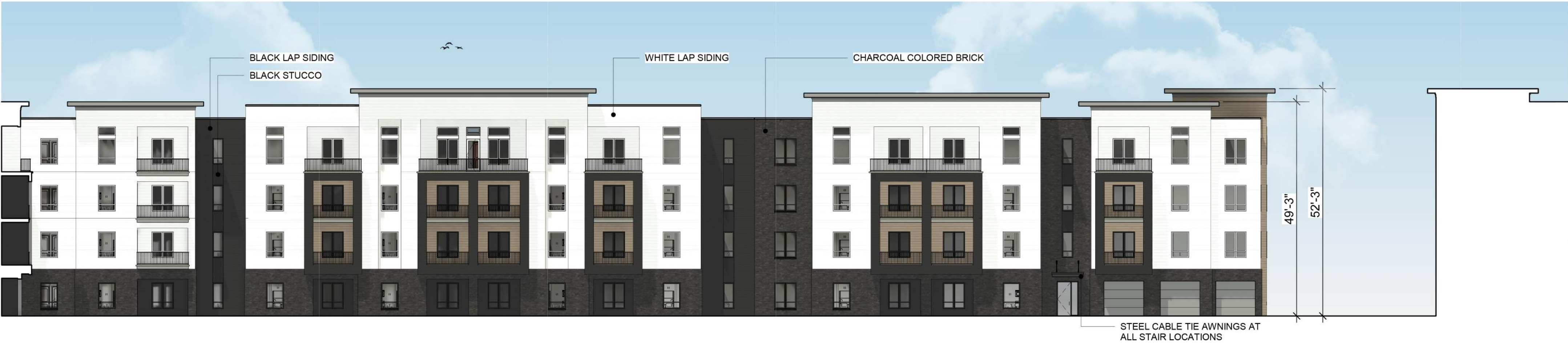
1 TYP. COURTYARD ELEVATION - 1ST FLOOR UNITS 1/16" = 1'-0"
