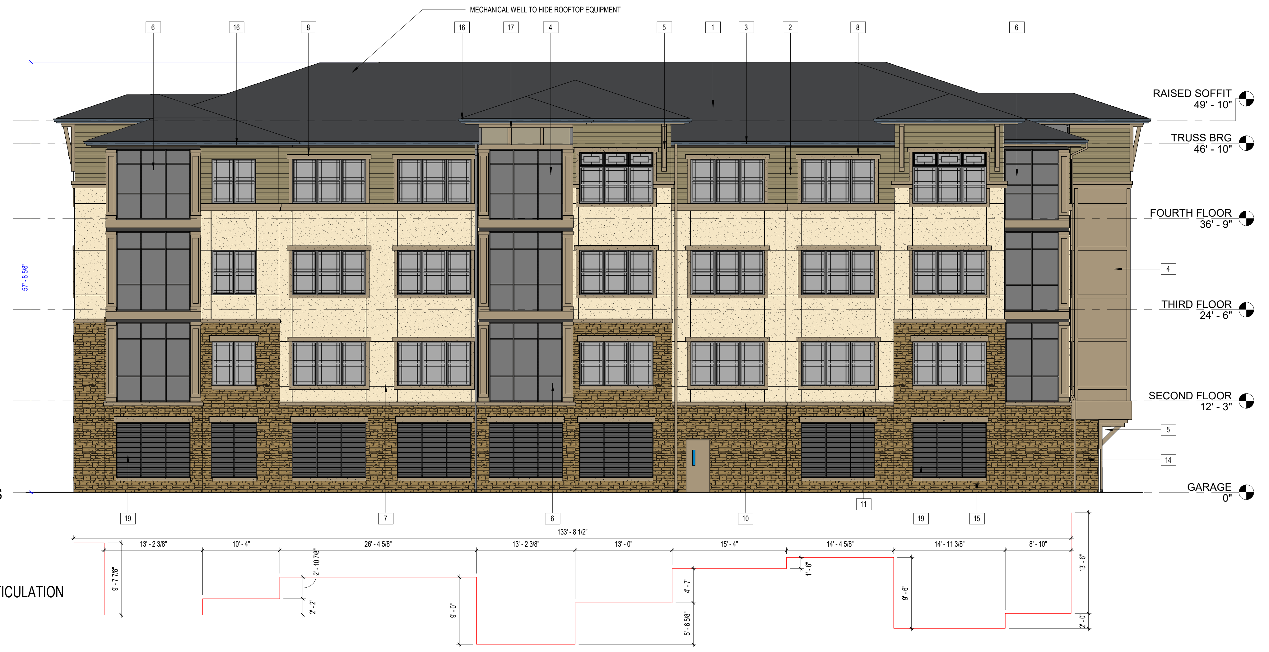
1 WEST ELEVATION - PDP 1/8" = 1'-0"
