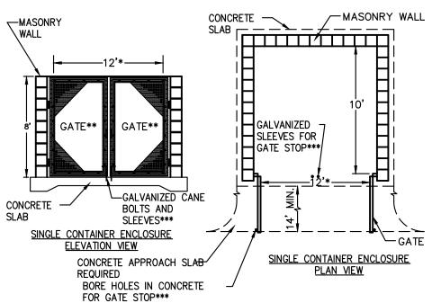
\* MINIMUM 12' CLEARANCE MUST BE PROVIDED BETWEEN GATE HINGES, POLES, POSTS, ETC. TO ALLOW FOR SOLID WASTE TRUCK ACCESS. \*\* SOLID STEEL OPAQUE GATE OR STEEL FRAMED SEMI-OPAQUE GATE WITH A SCREEN MESH MATERIAL APPROVED BY THE DIRECTOR THAT PROVIDES AN APPROPRIATE VISUAL BARRIER. \*\*\* OR OTHER APPROVED MECHANISM FOR SECURING THE GATES OPEN AND
