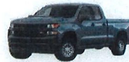
Cab "C" 4 full size doors, front hinged front & back seats (Crew Cab)
