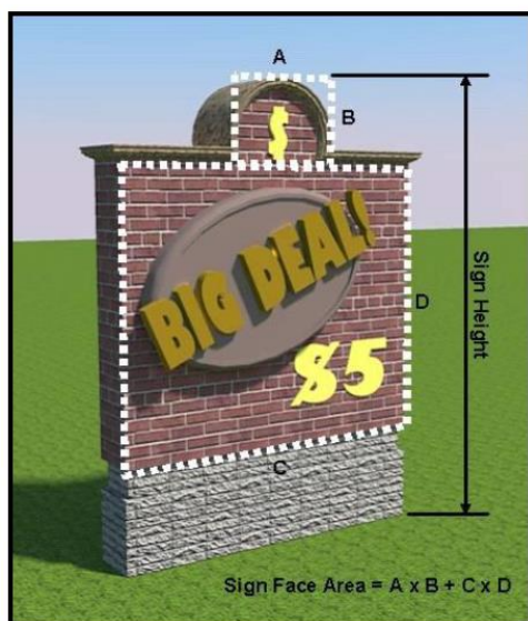
Measuring Sign Face and Sign Height
