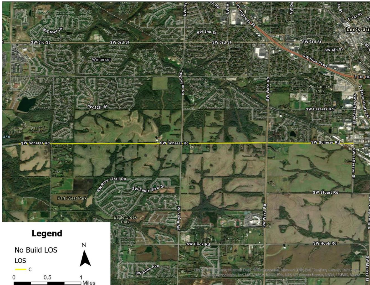
Figure 13 – Projected 2055 No Build LOS
