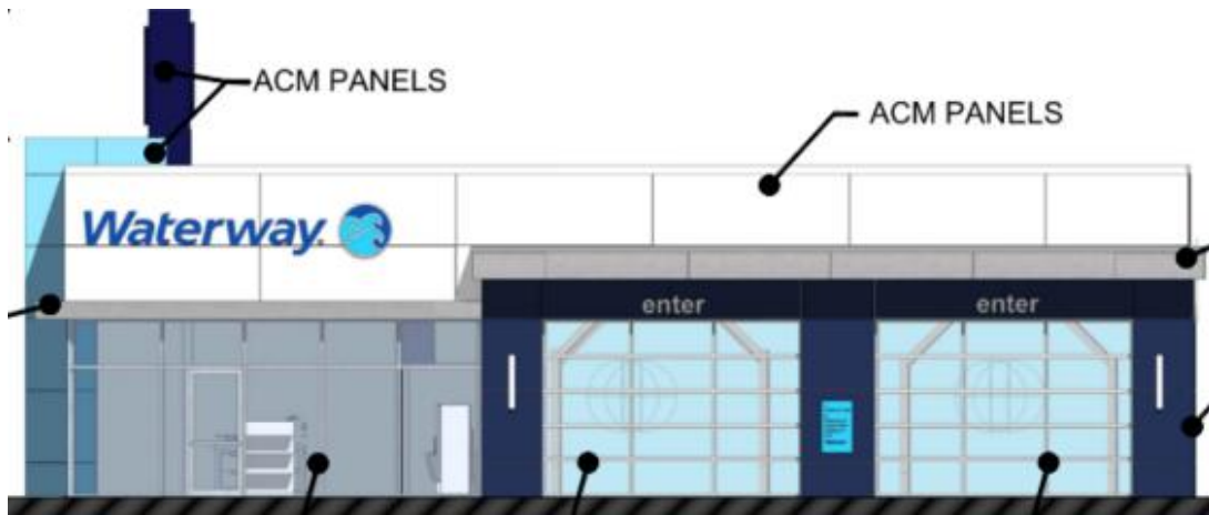
Figure 5 - West building elevation.
