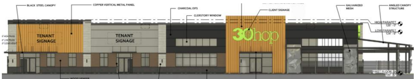
Figure 3 - Proposed Lot 13 front building elevation. Metal panel system shown in copper penny color.
