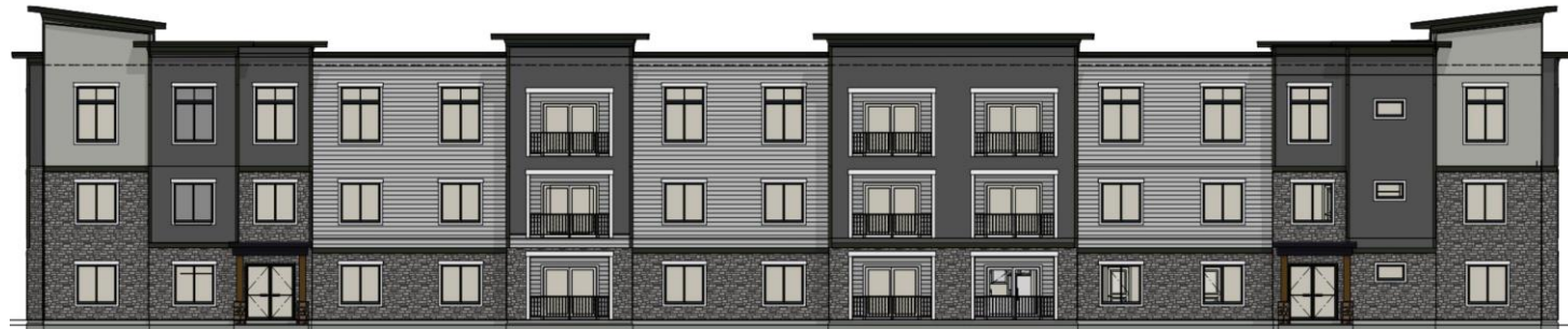
Materials: cement siding, stucco and stone
