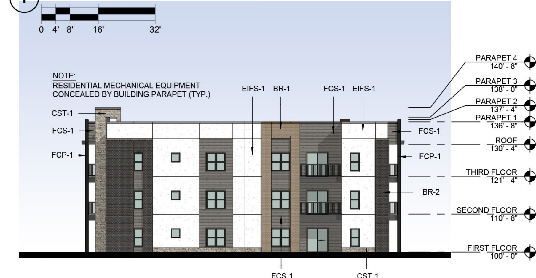
2 PARTIAL EAST ELEVATION (S)
