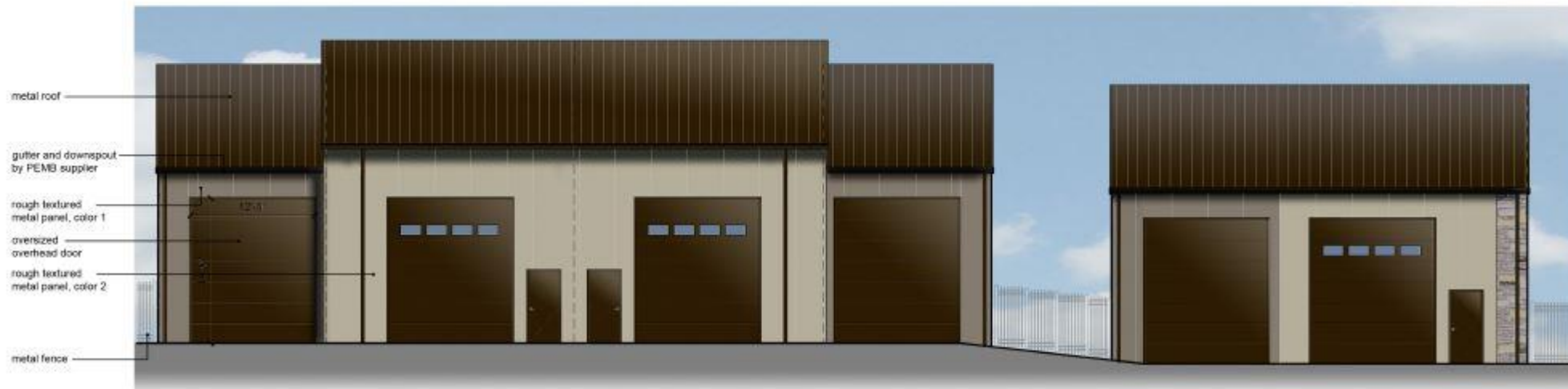
4 North Elevation (interior facing) - Bldg 7 scale: 1/8" = 1'-0"
