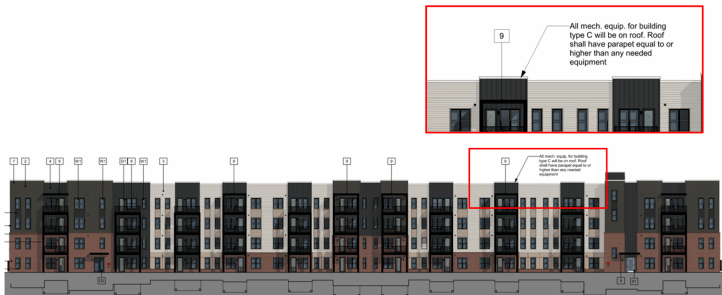
Figure 2 – Building Type "C" elevation showing the revised parapet height to screen rooftop equipment
