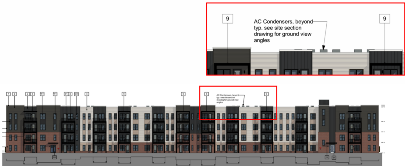
Figure 1 – Original Building Type “C” elevation showing the height of the rooftop equipment in comparison to the height of the parapet.
