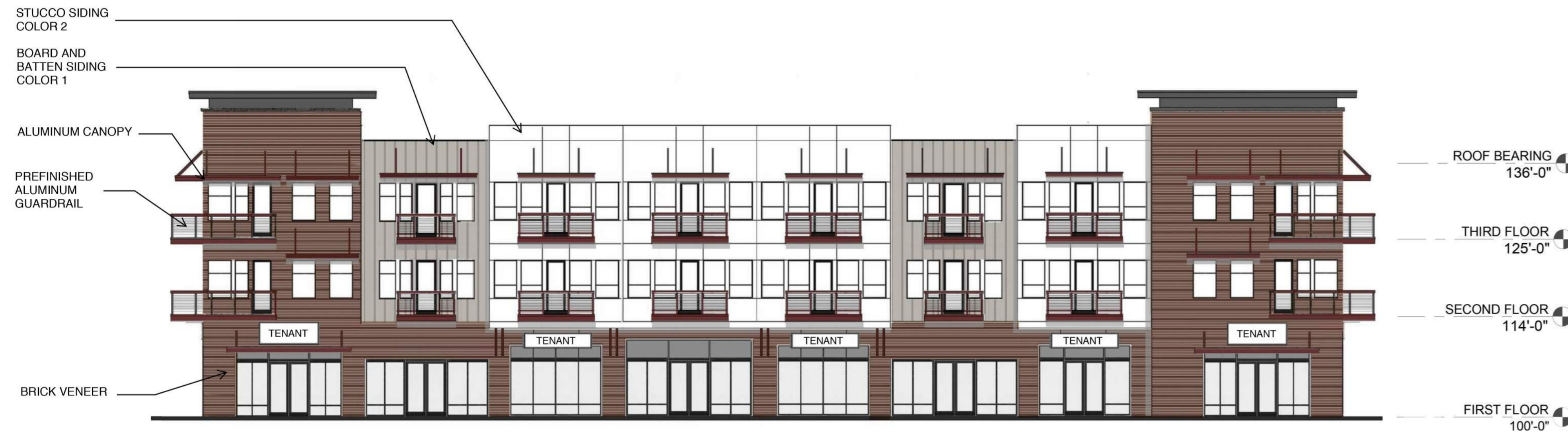
3 BLDG 4 NORTH ELEVATION 3/32" = 1' - 0"
