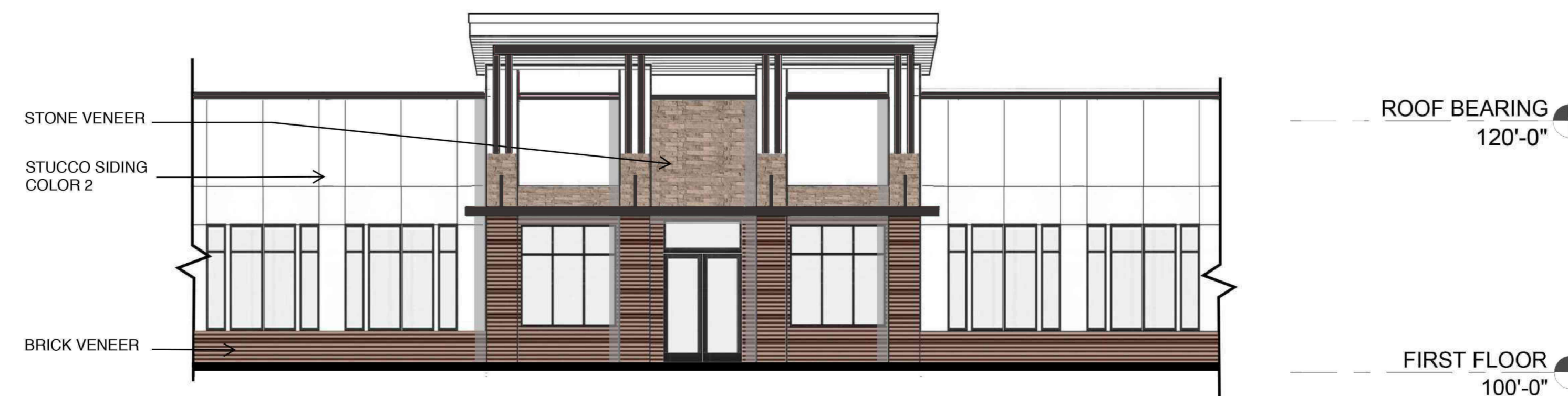
1 TYPICAL ENTRY NORTH ELEVATION 1/8" = 1' -0"
