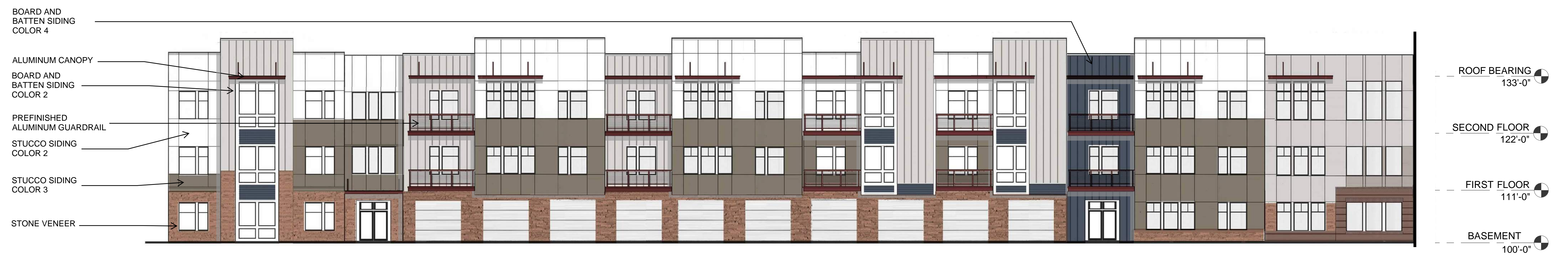
1 BLDG 1 WEST ELEVATION 3/32" = 1' - 0"
