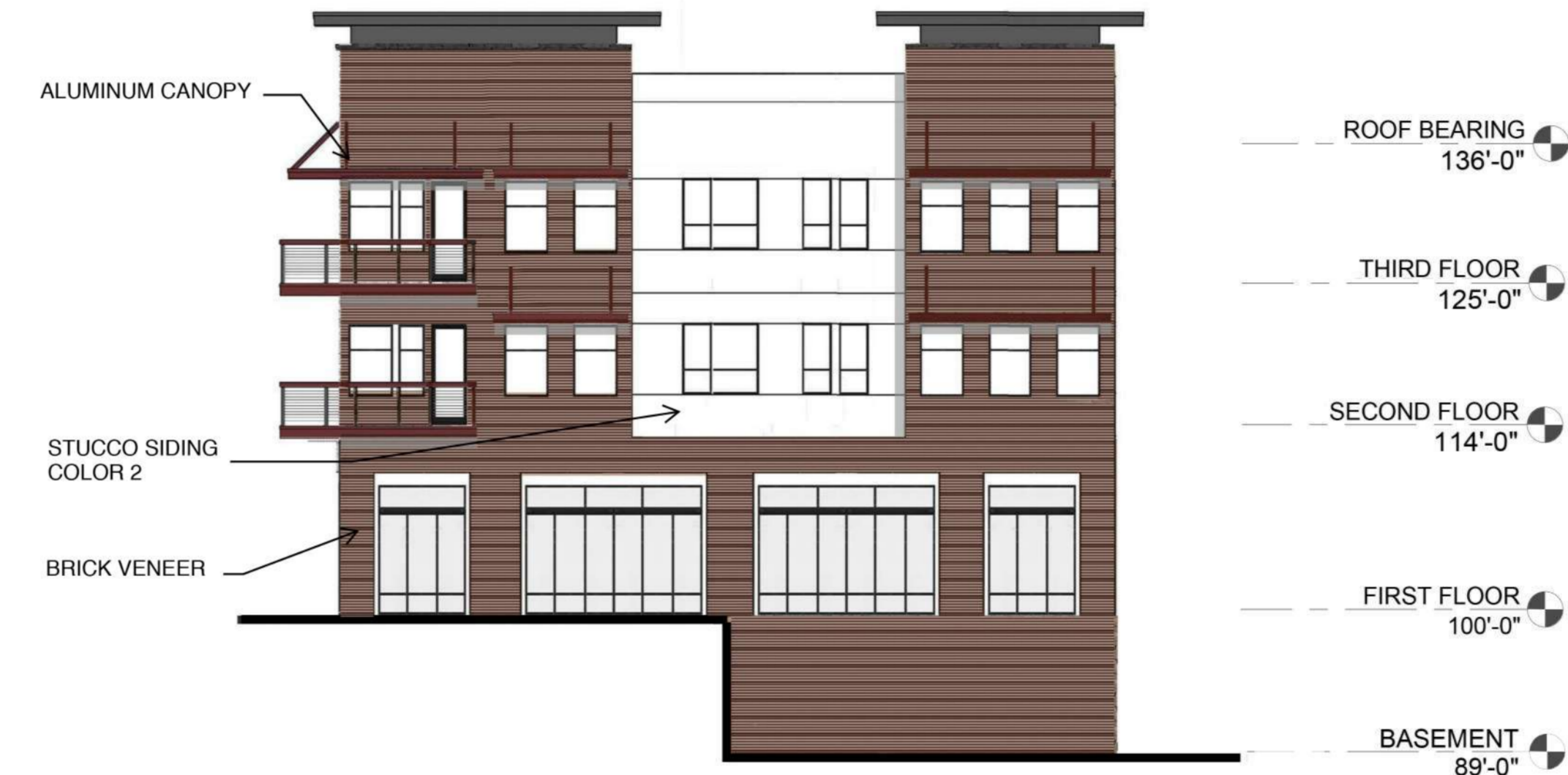
2 BLDG 4 SOUTH ELEVATION 3/32" = 1' - 0"
