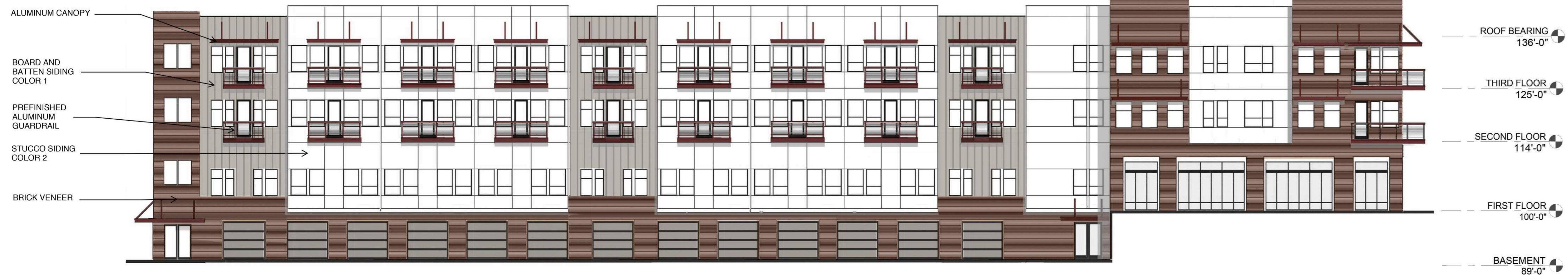
1 BLDG 4 EAST ELEVATION 3/32" = 1' - 0"
