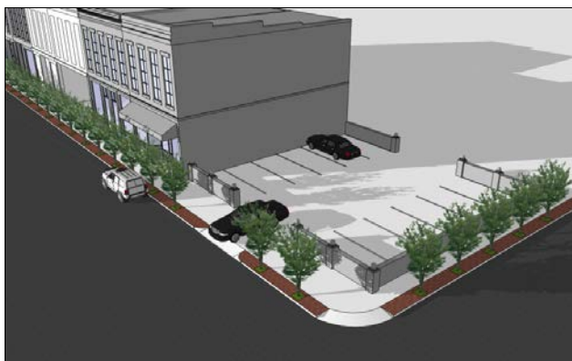
Corner parking lots shall not have the edges defined through a masonry wall or other structure. Landscaping may be used in conjunction with the solid screen wall.
