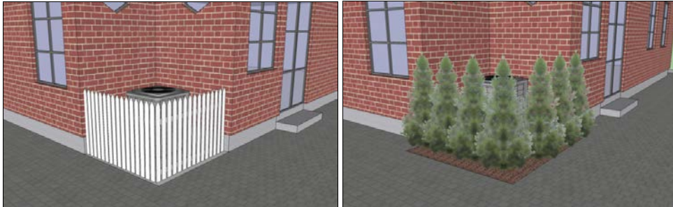
HVAC units and condensers at rear facades shall be screened through fencing or landscaping. Units should have 36" of clearance to allow for maintenance and servicing.
