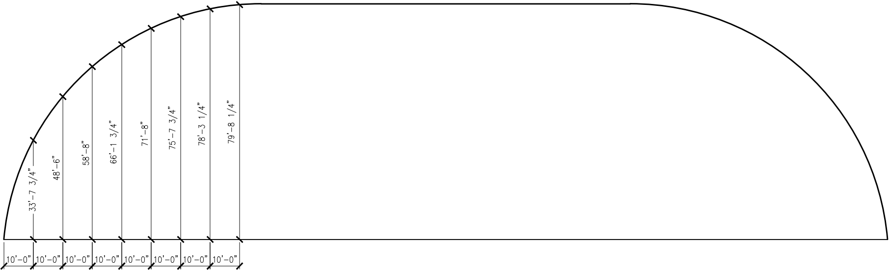
02 DOME PROFILE HEIGHTS SCALE: 1/16"=1'-0"
