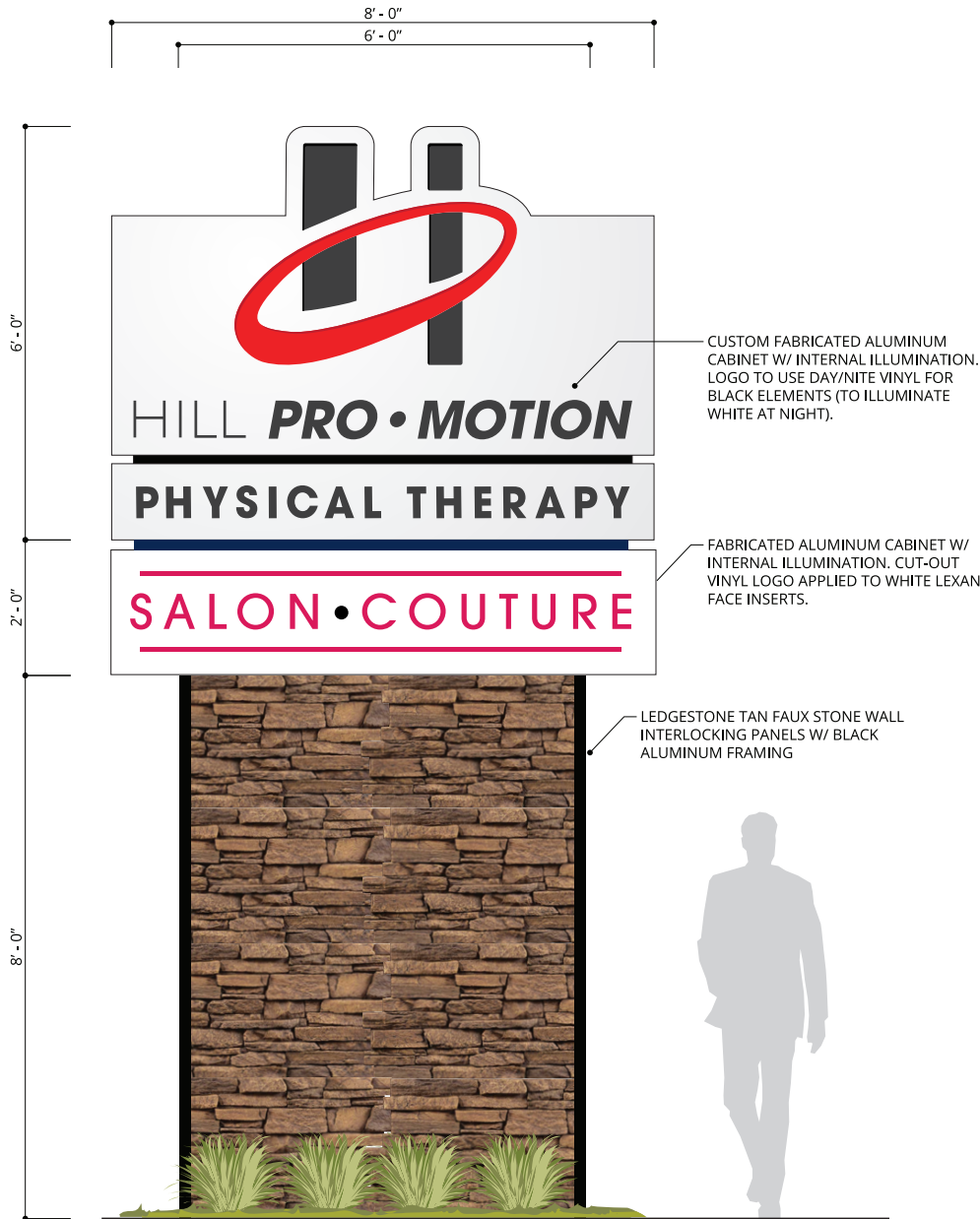
Illuminated Pole Sign Scale: 1/2" = 1' - 0"
