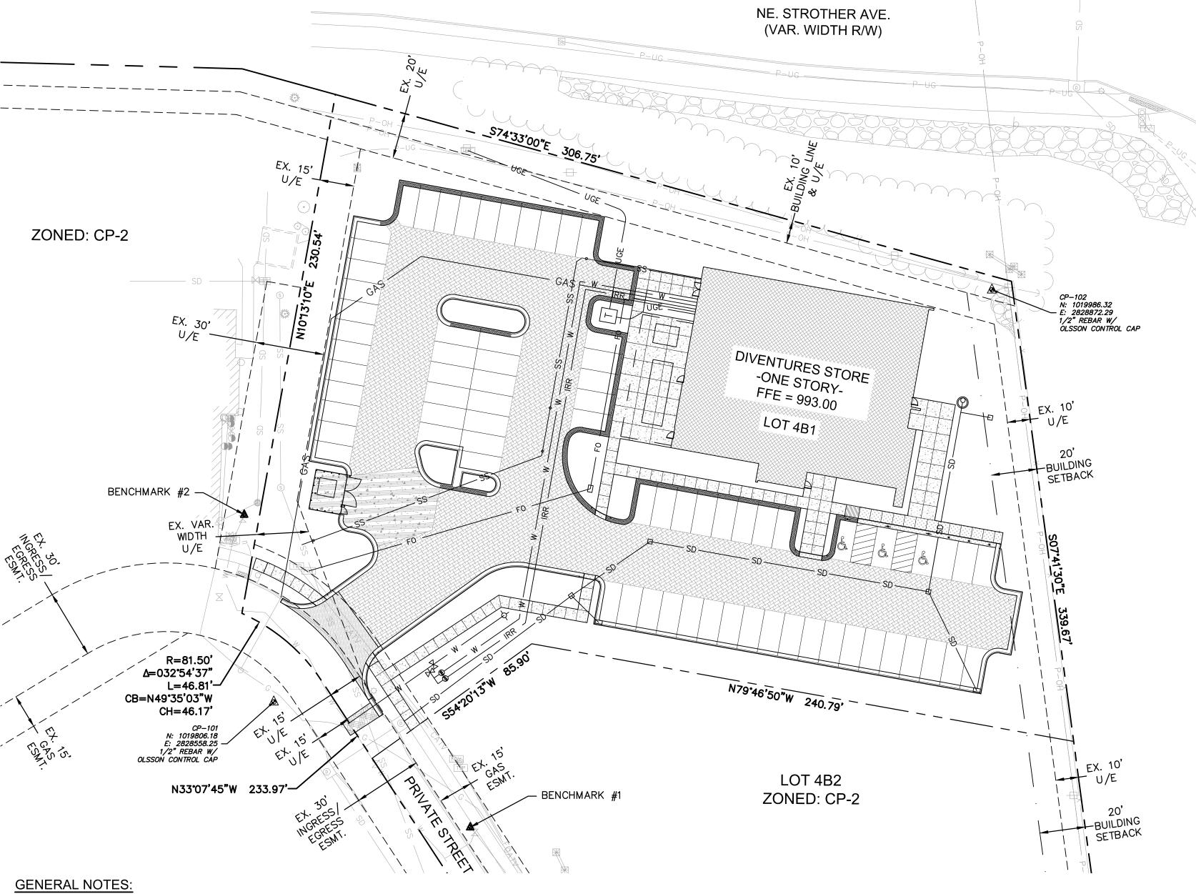
16. CONTRACTOR SHALL FINISH GRADE SLOPES AS SHOWN NO STEEPER THAN 1 FOOT VERTICAL IN 3 FEET HORIZONTAL.
