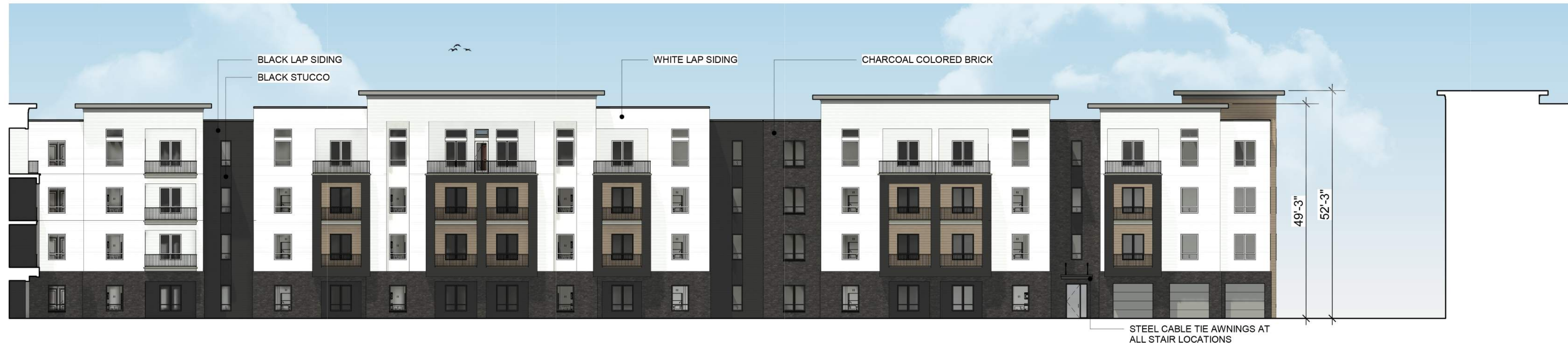
1 TYP. COURTYARD ELEVATION - 1ST FLOOR UNITS 1/16" = 1'-0"
