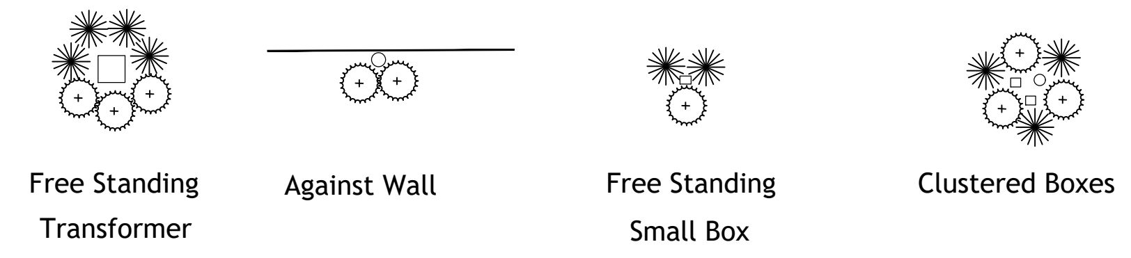
Typical Utility Box Screening Details No Scale
