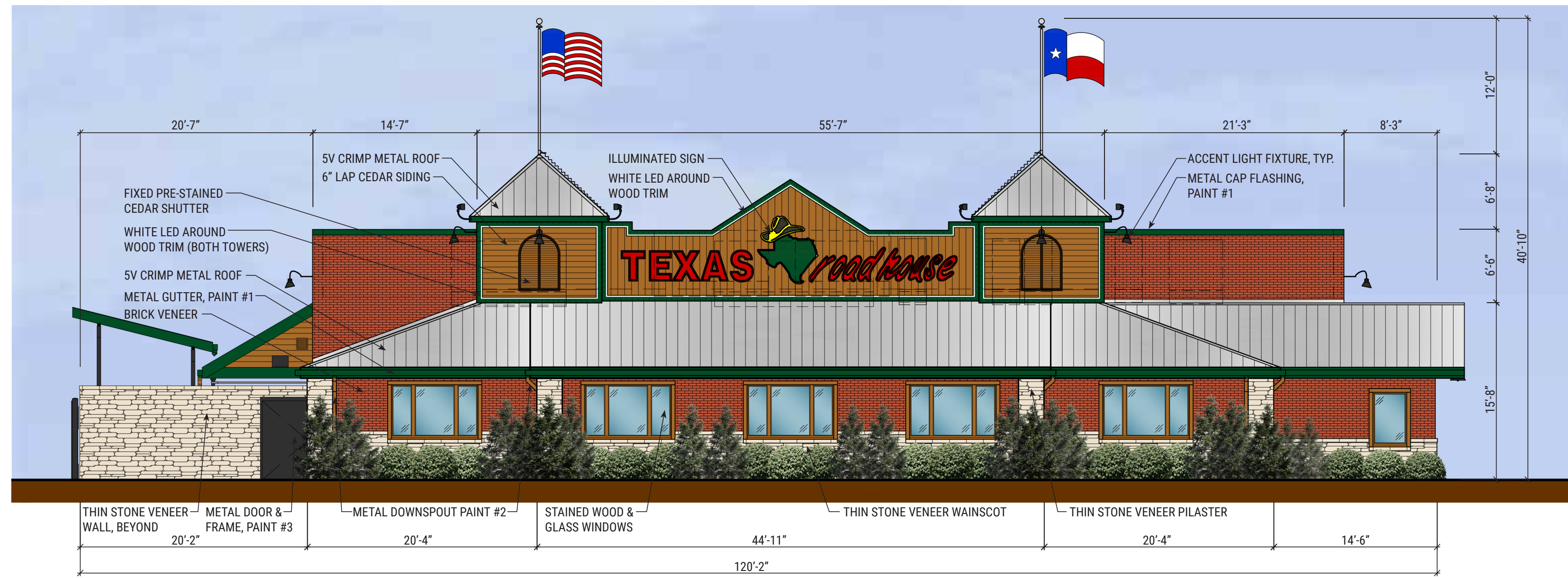
FRONT ELEVATION (WEST)
