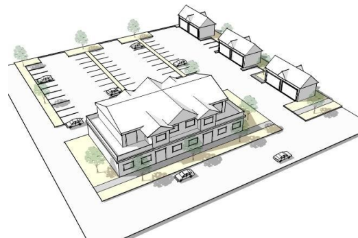
Multi-family parking located behind primary structure
